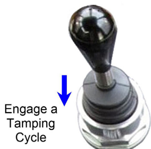
Figure 6-12: Joystick Motion for the Tamping Cycle
