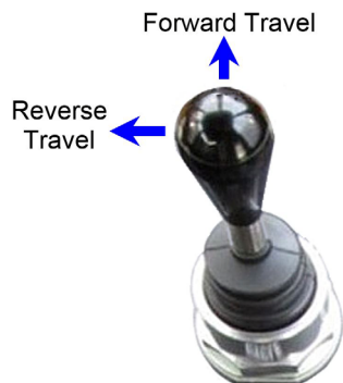
Figure 6-11: Joystick Motions for Machine Travel
