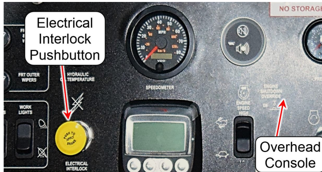
Figure 5-25: Electrical Interlock Button on the Overhead Console
