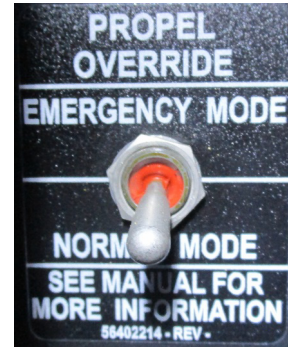
Figure 5-21: Propel Override Switch Inside Cabinet
