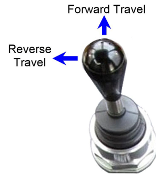
Figure 6-9: Joystick Motions for Machine Travel
