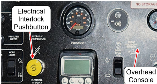
Figure 1-4: Electrical Interlock Pushbutton
