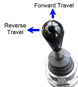
Figure 6-10: Joystick Motions for Machine Travel
