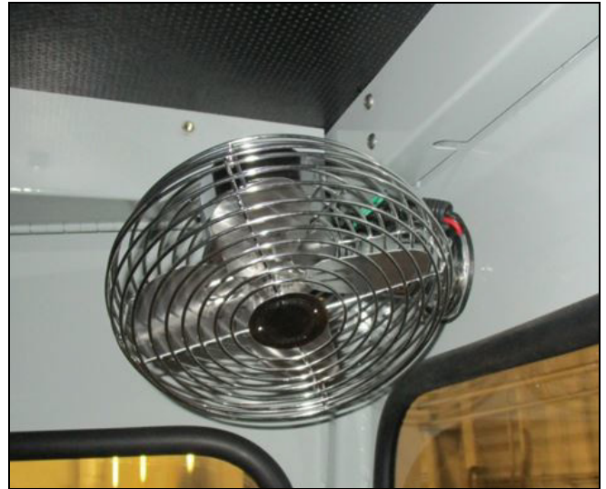
Figure 5-27: Ceiling Fan in the Cab
