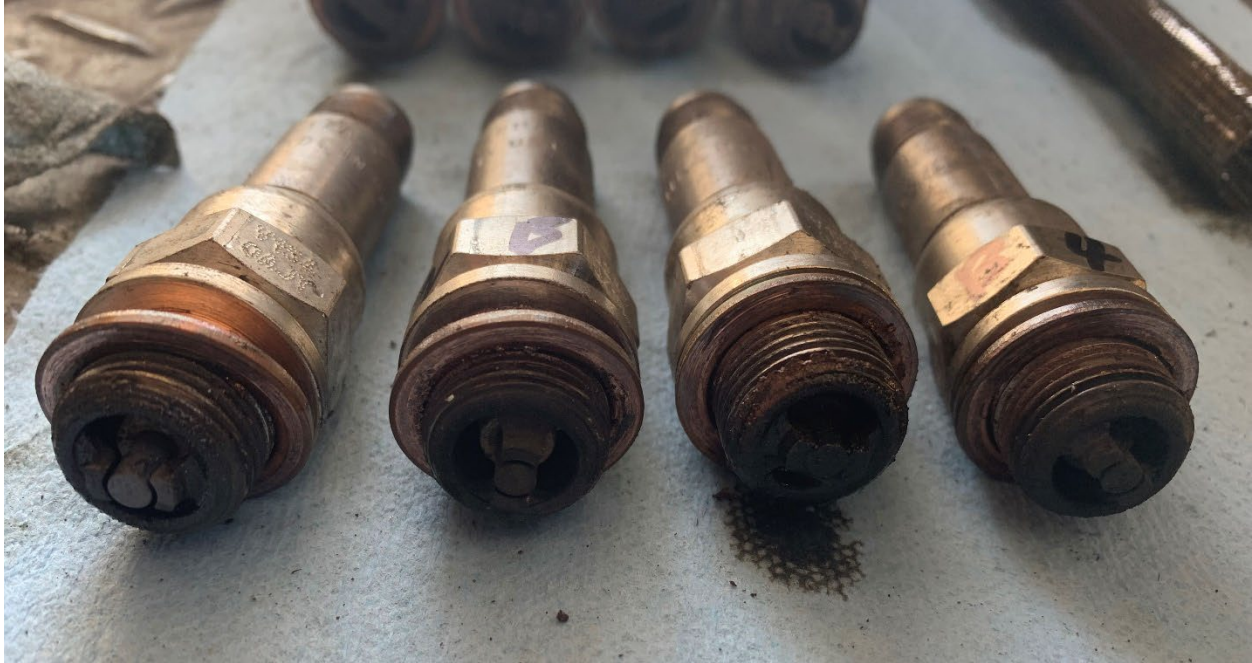
Figure 18. Bottom Spark Plugs
