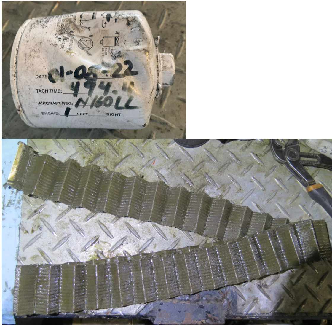
Figure 26. View of oil filter housing and filter.
