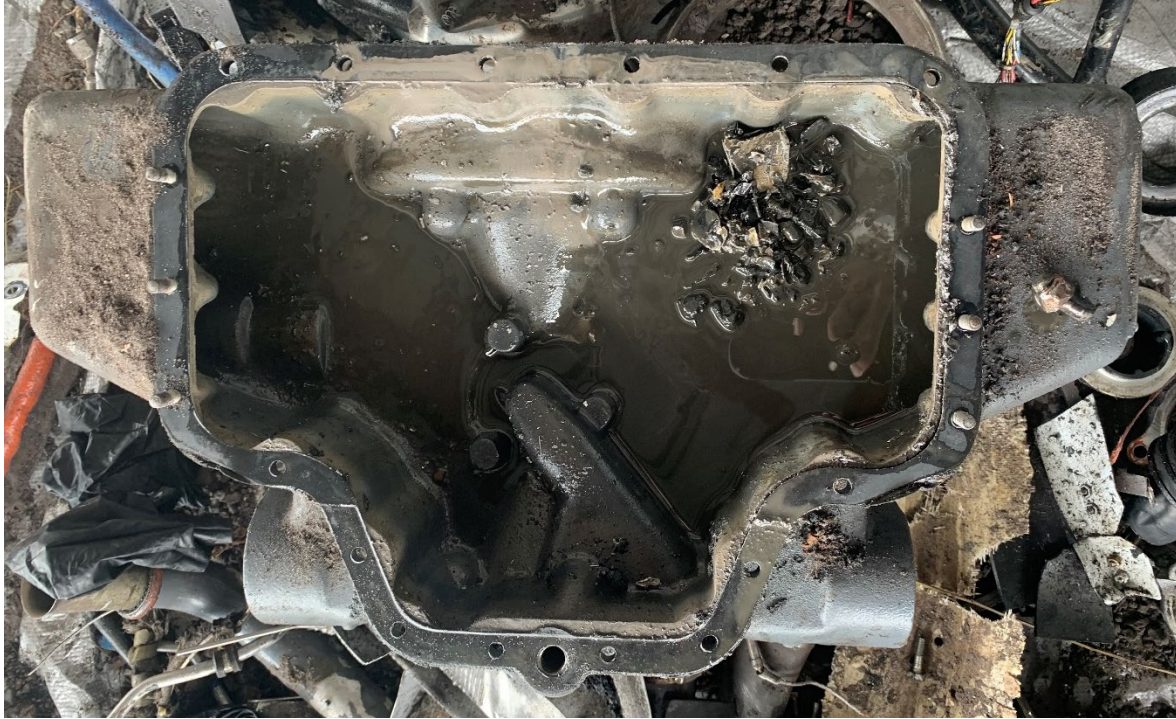
Figure 27. View of oil sump and debris in the sump.
