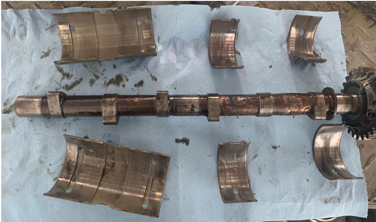
Figure 13. View of camshaft and main journal bearings. From left to right - front main bearing, center main bearing, rear main bearing.
