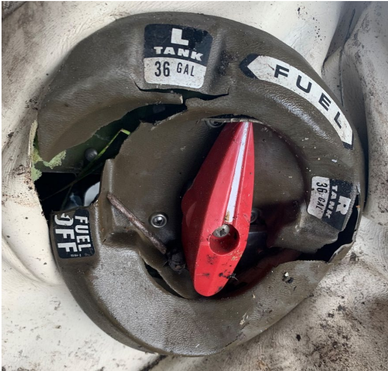
Figure 8. View of fuel selector as found.
