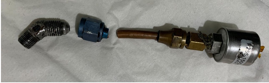
Figure 30. View of oil sensor line retained for further examination.
