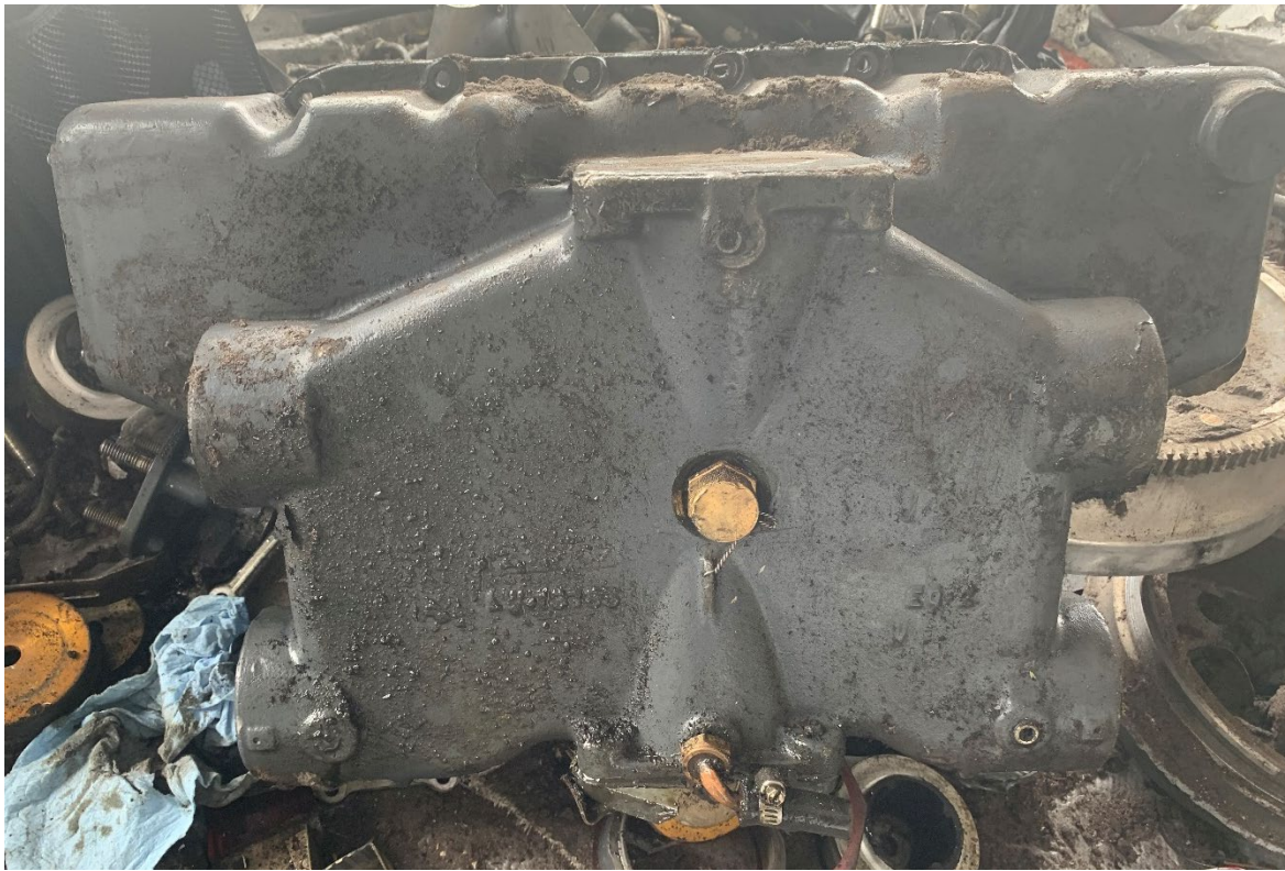
Figure 28. View of oil drain plug safety wired into the oil sump.
