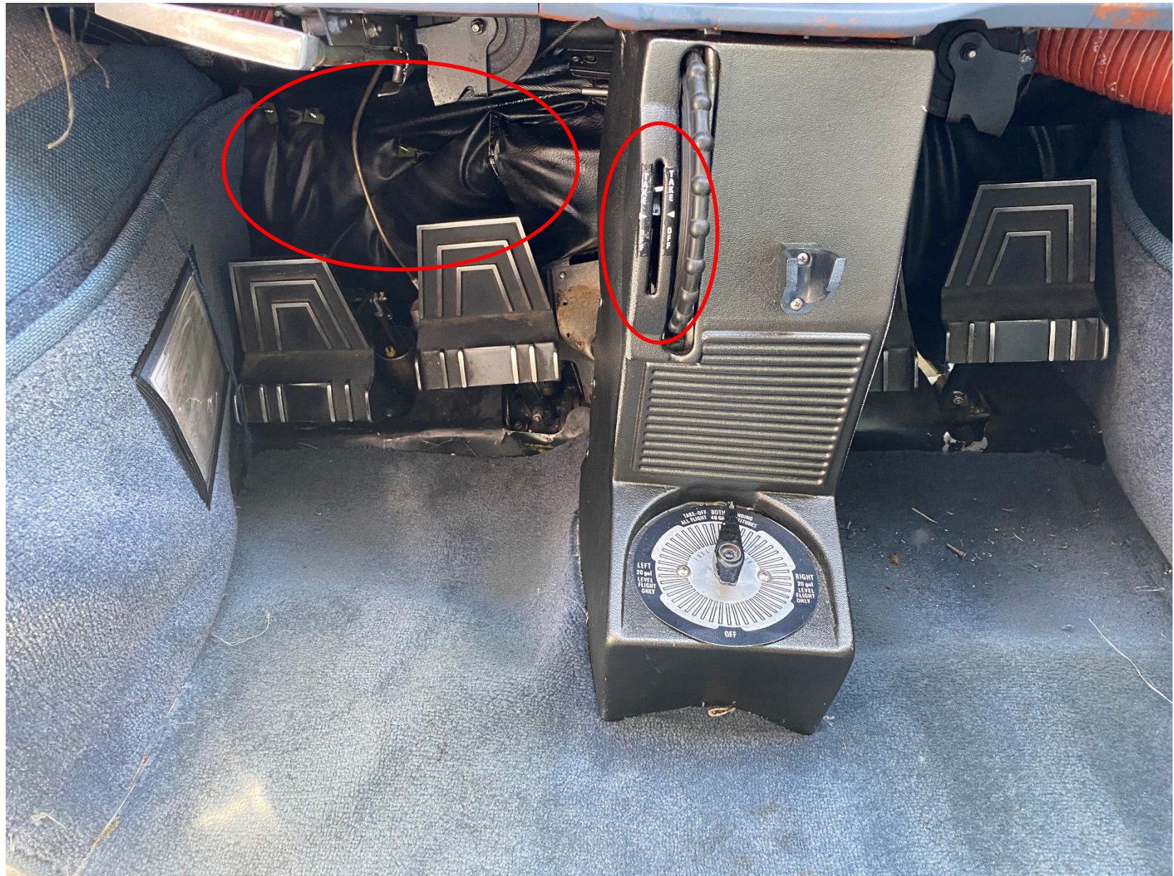
Airplane – View of Interior Damage and Pitch Trim Indicator (courtesy FAA)
