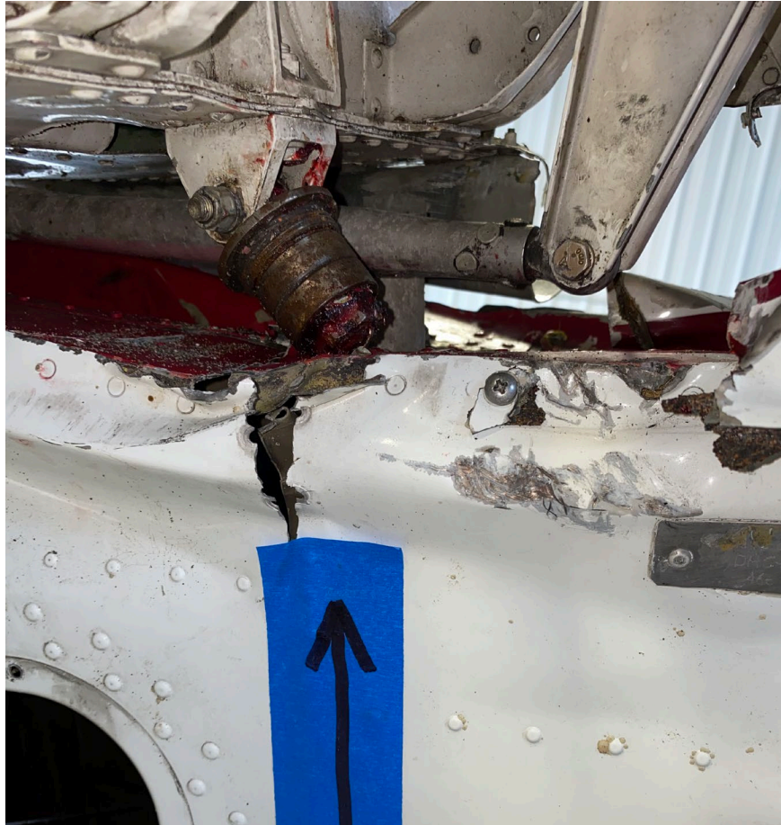
Photograph 5 - Trim Actuator Upper Mount (with Actuator Top Eye end and Bearing Assembly Attached)
