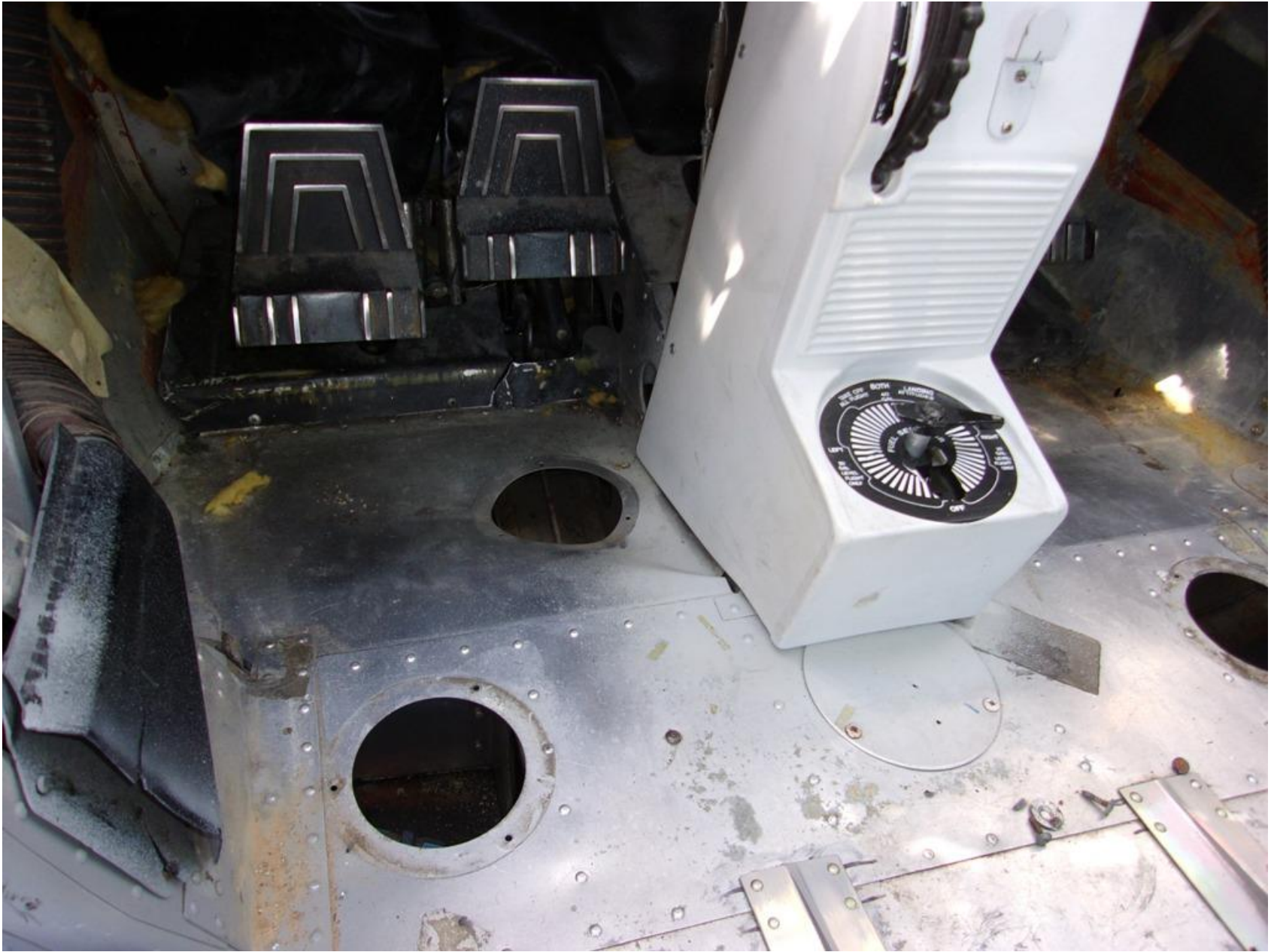
Photo 2 – Lower Fuselage Structural Damage
