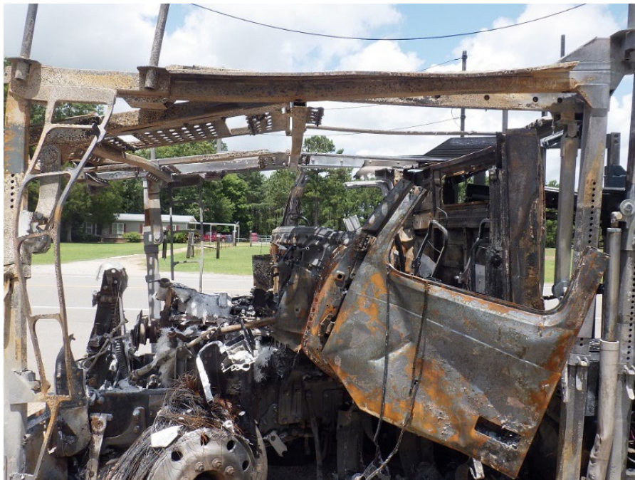
Figure 1. Driver side view of the Volvo truck-tractor showing fire damage, deformation of the firewall, driver door, and aft portion of the cab.
