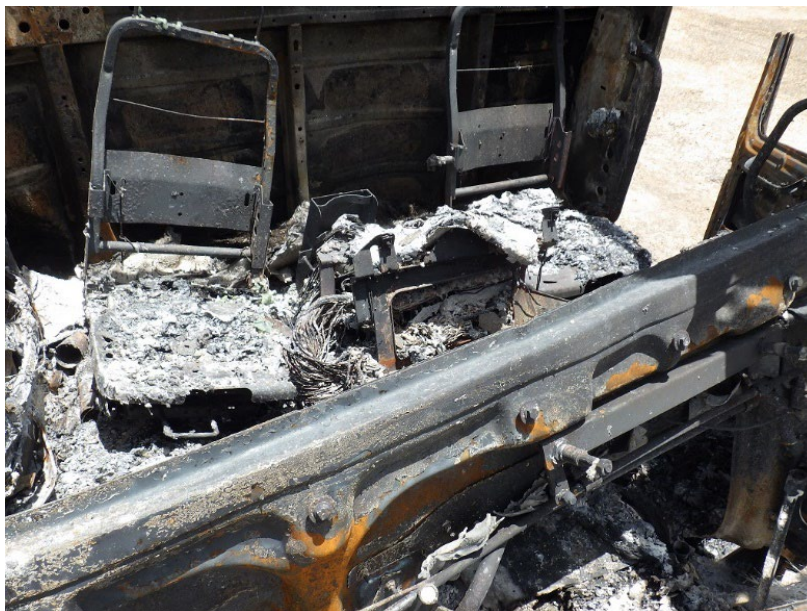
Figure 2. View from the firewall looking aft of the Volvo truck-tractor showing fire damage, the driver and passenger seat frames, and deformation of the passenger seat.
