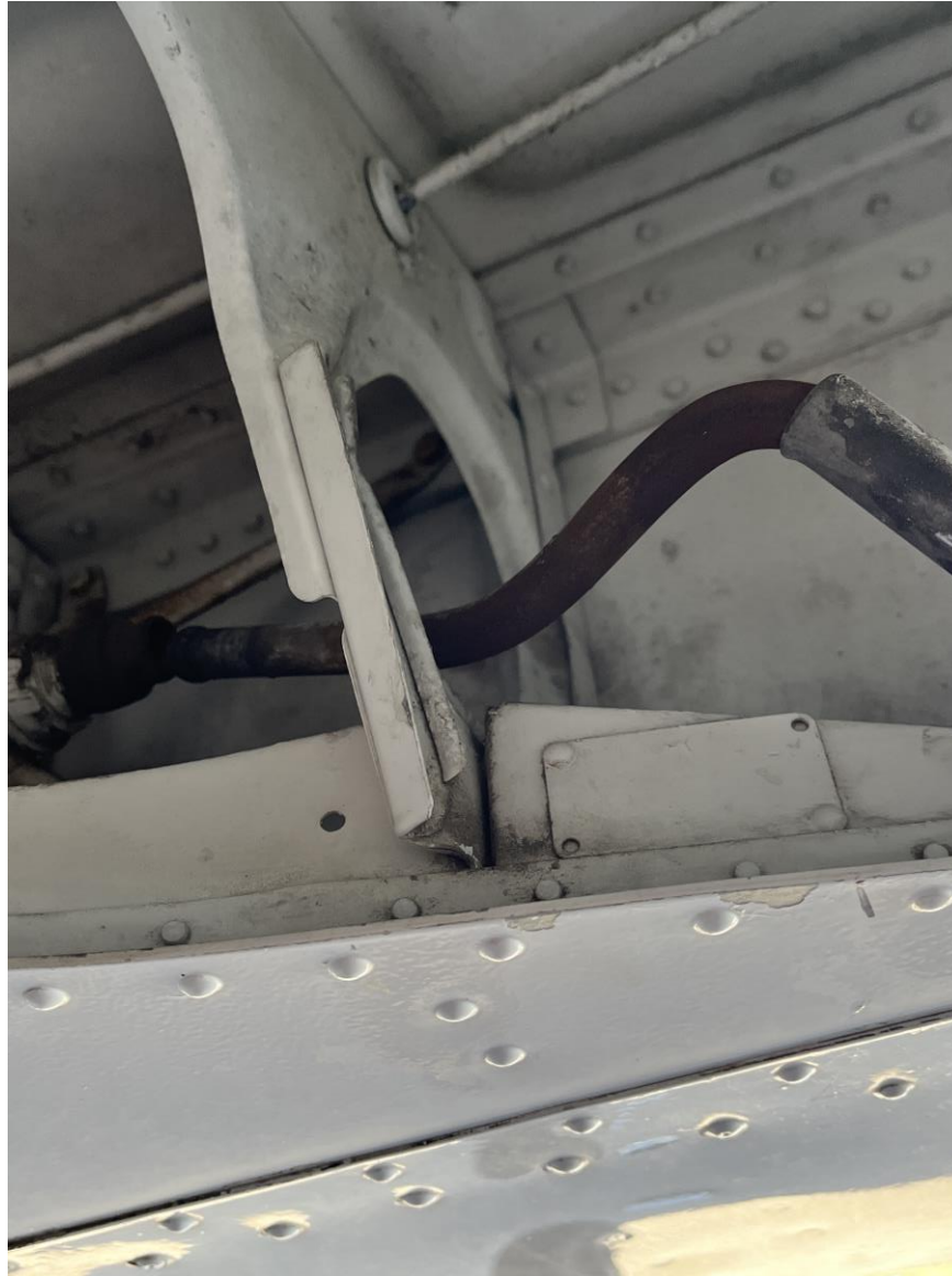
Photograph 4 - Bent right main landing gear push rod (Courtesy of A&P mechanic)
