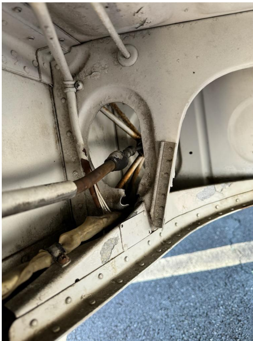
Photograph 6 - Bent left main landing gear push rod (Courtesy of A&P Mechanic)
