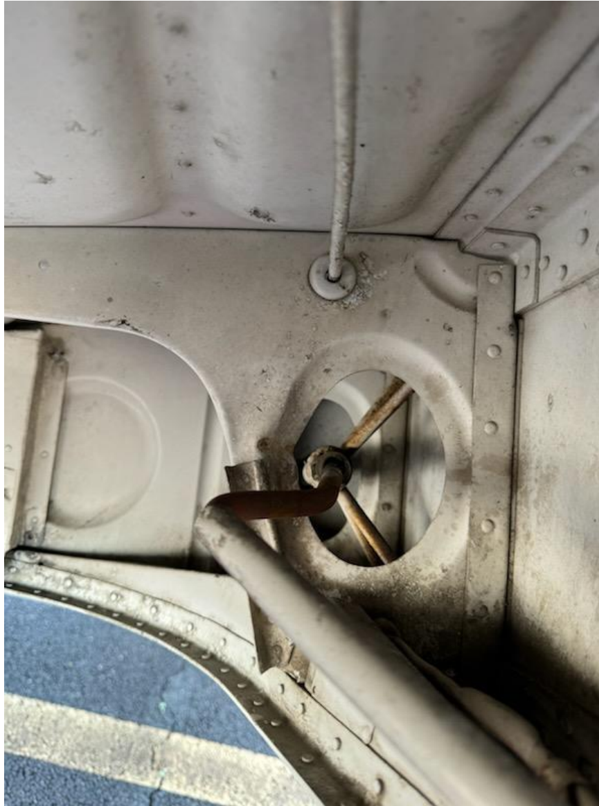
Photograph 5 - Bent right main landing gear push rod (Courtesy of A&P Mechanic)
