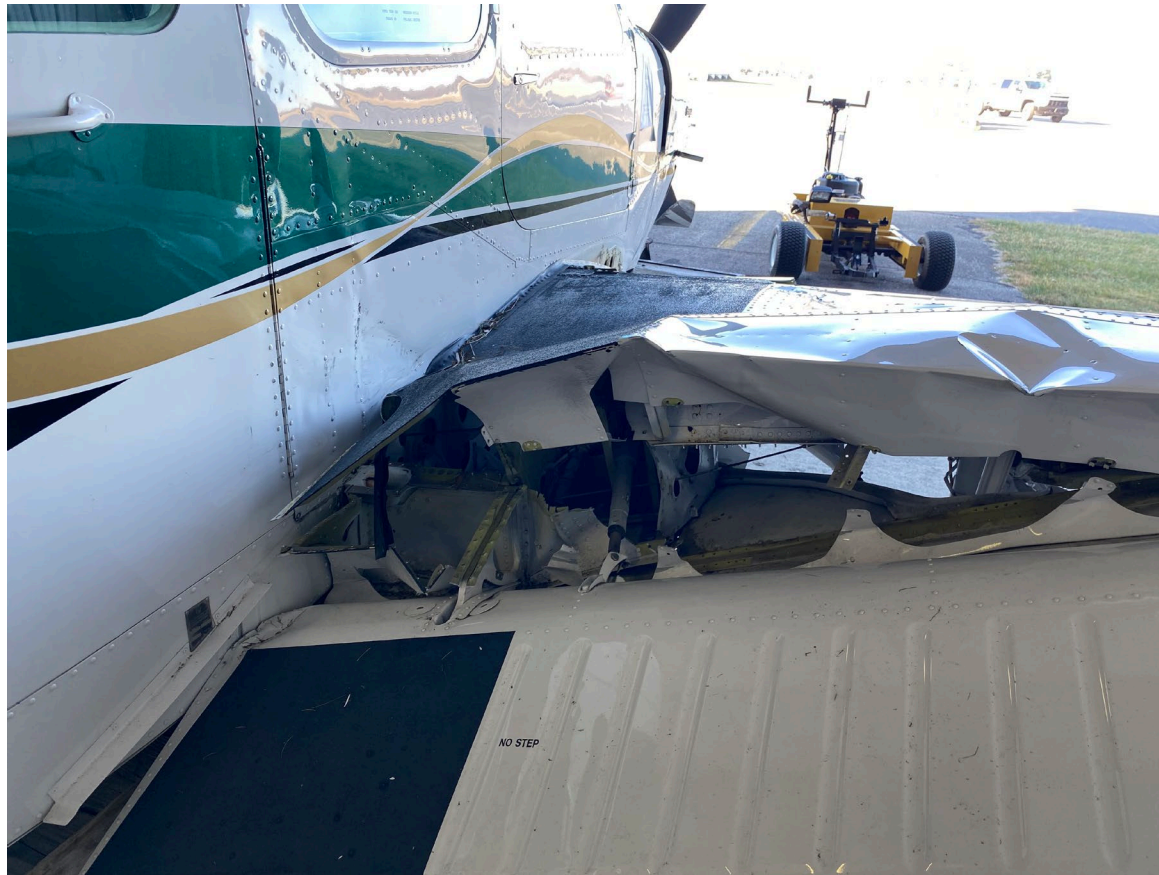
Photograph 3 - Damage to right wing (Courtesy of FAA)
