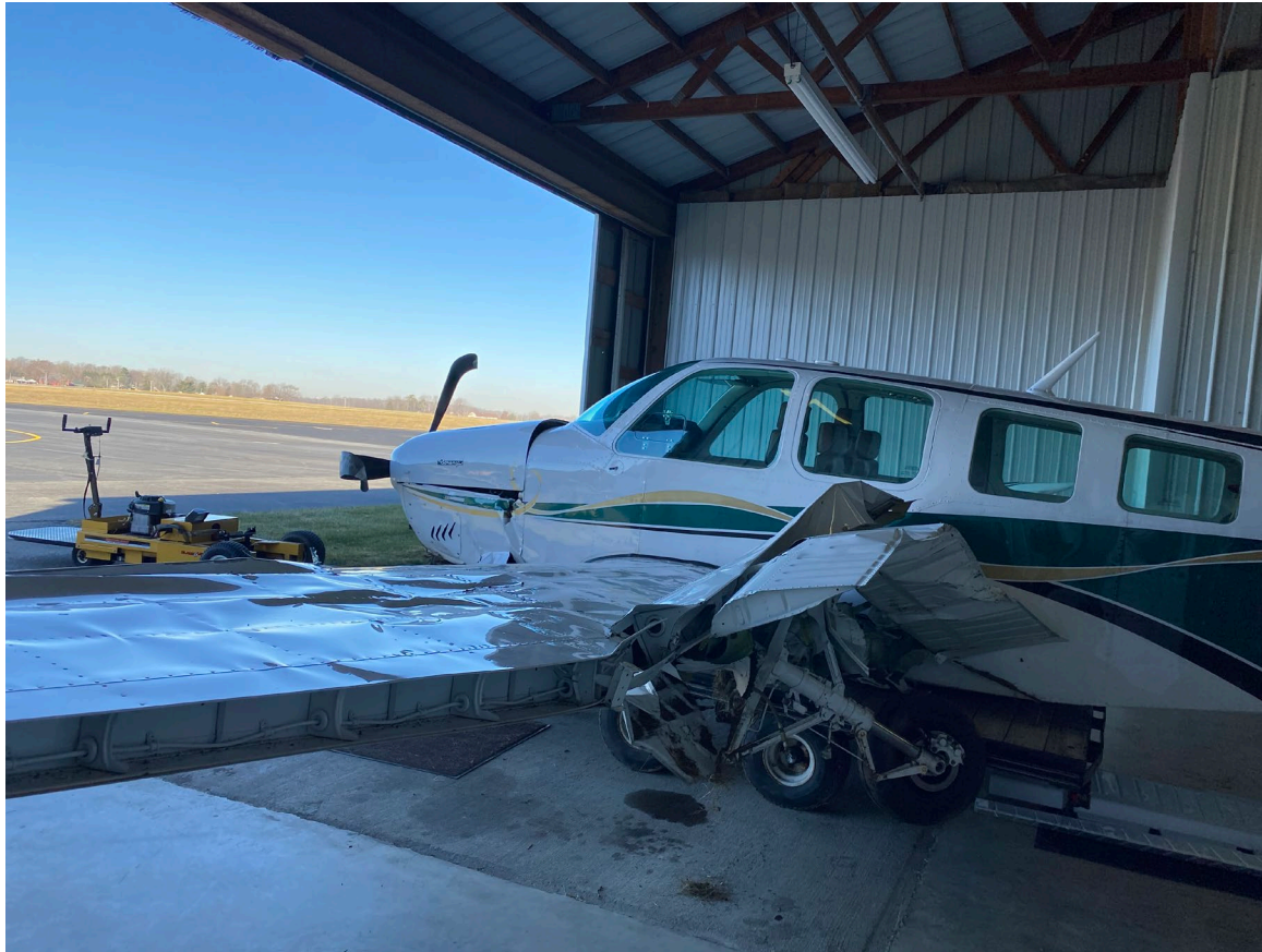
Photograph 2 - Damage to left wing (Courtesy of FAA)
