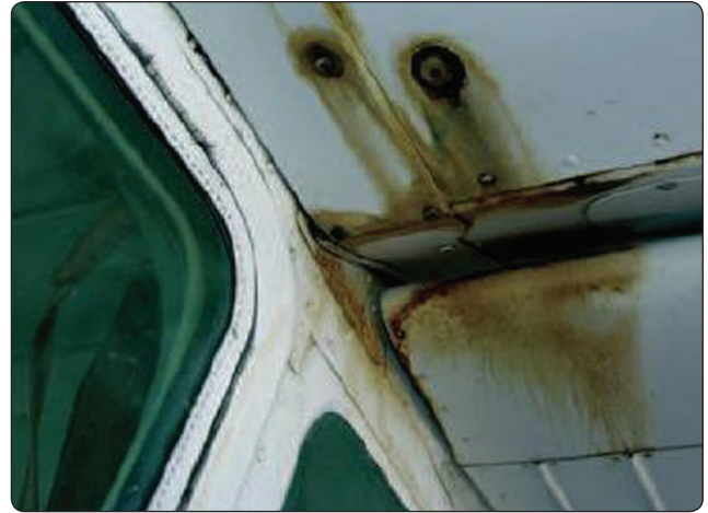
Figure 2-11. Evidence of fuel leakage can be found along rivet lines.
