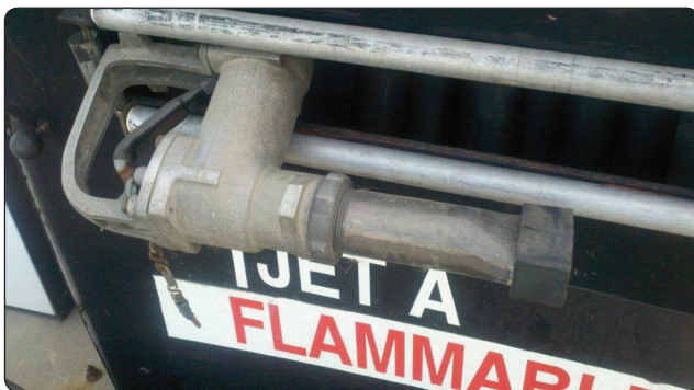
Figure 2-10. A jet fuel filler nozzle is flared at the end to prevent an inadvertent insertion into an AVGAS fuel tank.
