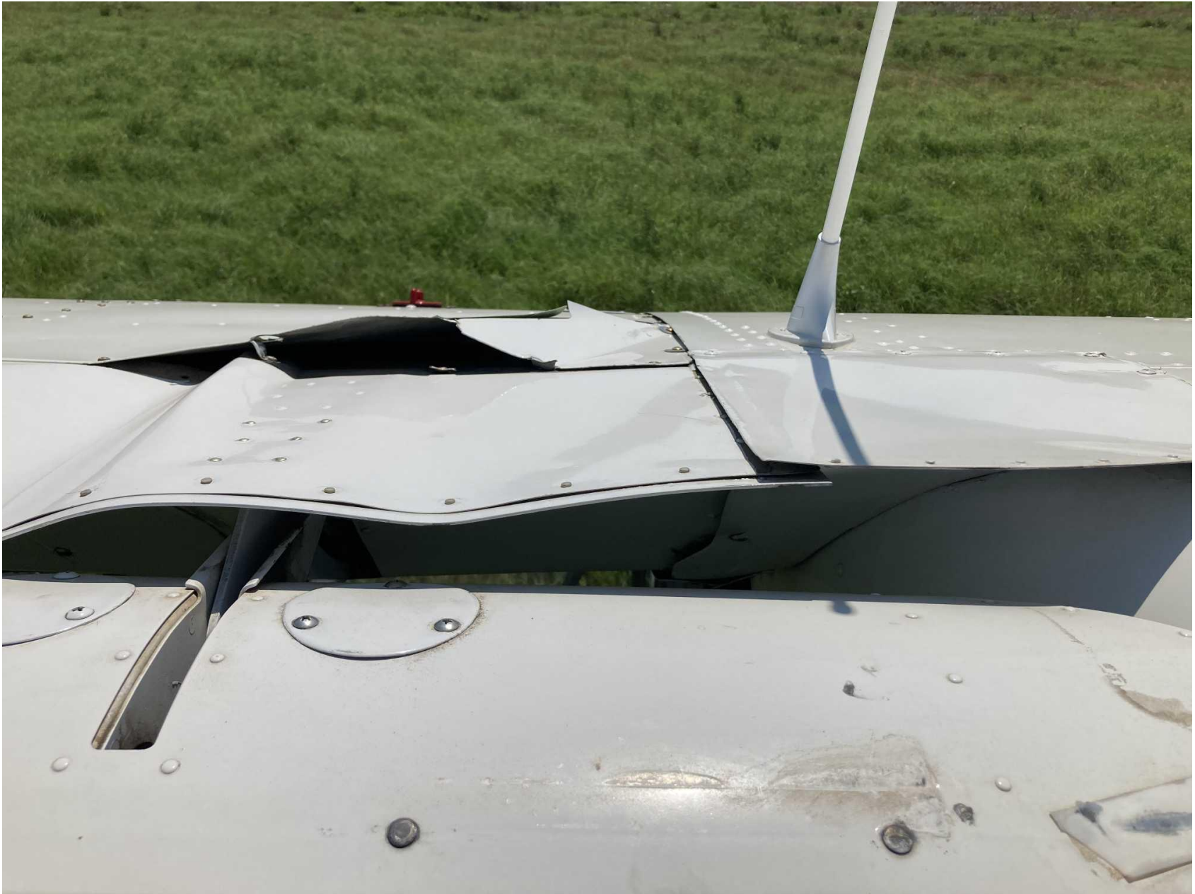
Photo 2 – Left Wing Rear Spar Damage (Photo Provided by Airplane Owner/Operator)
