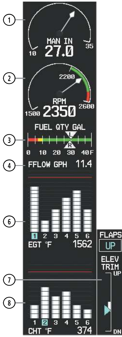
Figure 3-15 Lean Display (M20R - Normally Aspirated)
