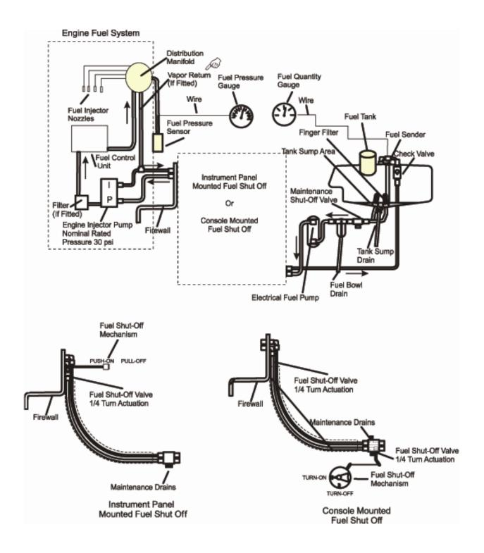
Figure 7.6 - Fuel System Schematic Diagram
