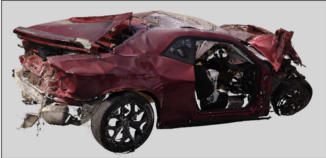
Figure 9: Screen capture image depicting colorized 3D point cloud of Dodge as viewed from right side of vehicle.
