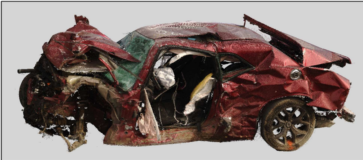
Figure 8: Screen capture image depicting colorized 3D point cloud of Dodge as viewed from left side of vehicle.
