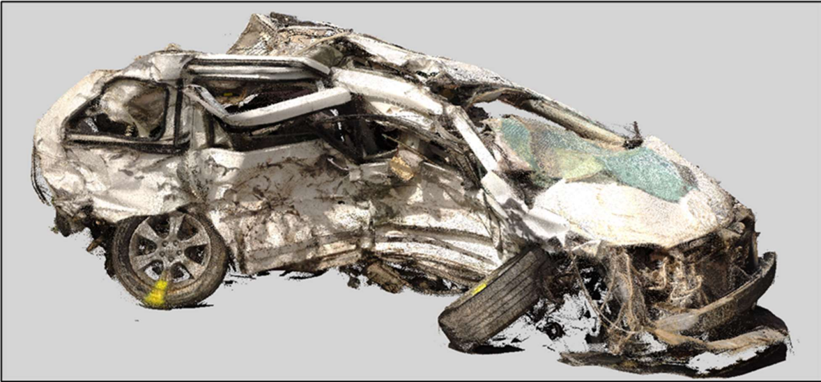
Figure 10: Screen capture image depicting colorized 3D point cloud of the Toyota as viewed from right side of vehicle.
