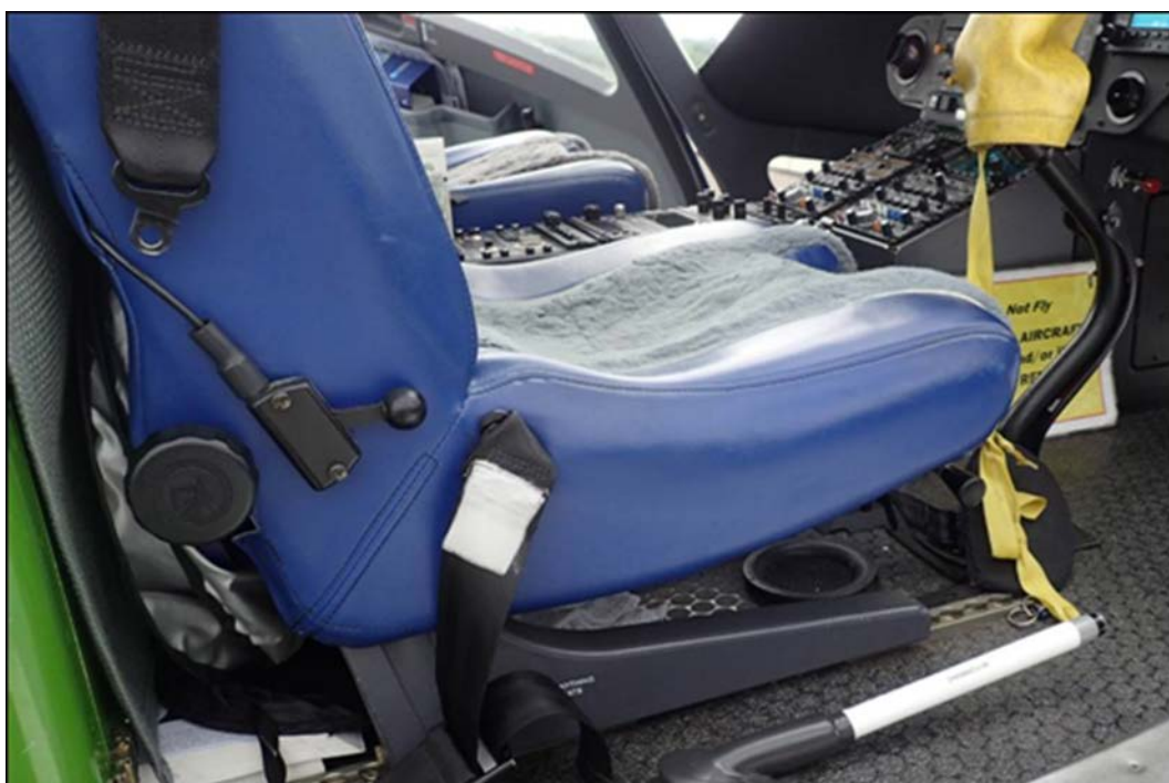
Figure 12 – View of the five-point restraint system and the inertia reel lock lever mounted on the outer right side of the seat, N145DU.
