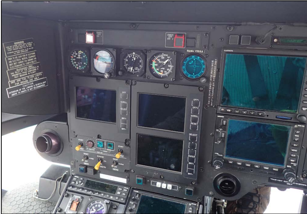
Figure 16 – Exemplar right seat view of the caution and warning unit in N145DU.
