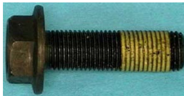
ZOH-T Bolt: flange head, dark in color, fine thread, may have thread patch as shown (M12x1.25x40).
