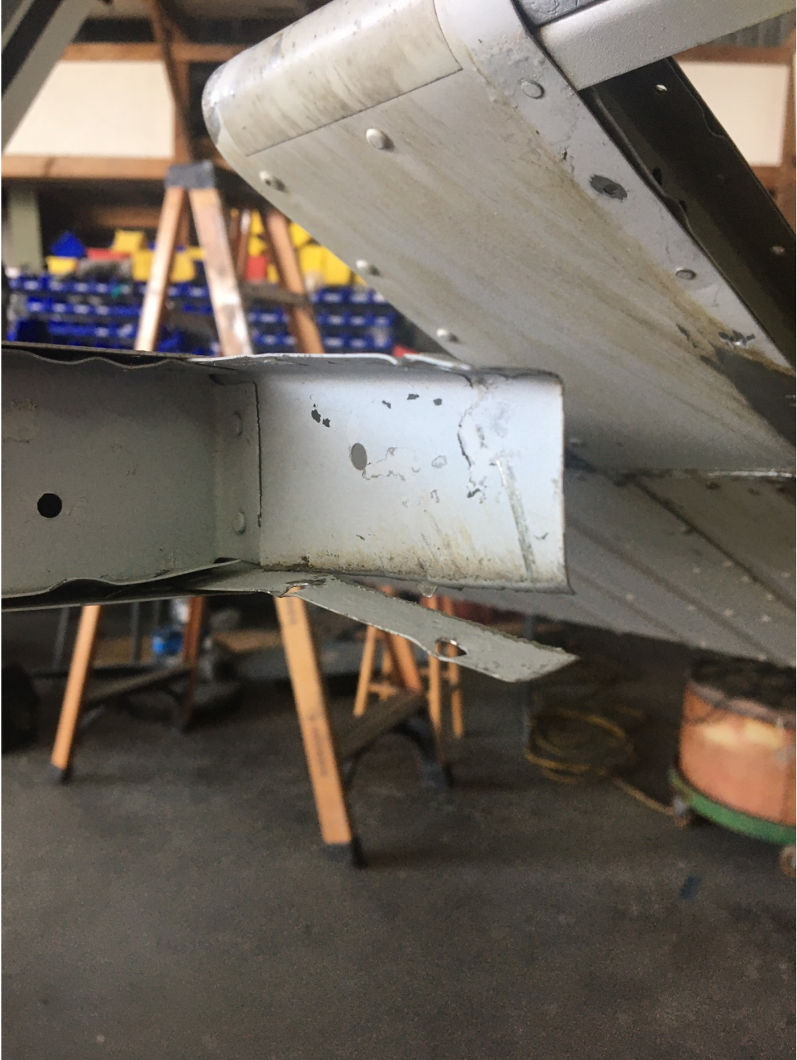
Figure 1 Damage to Left Side Horizontal Stabilizer Spar and Rib
