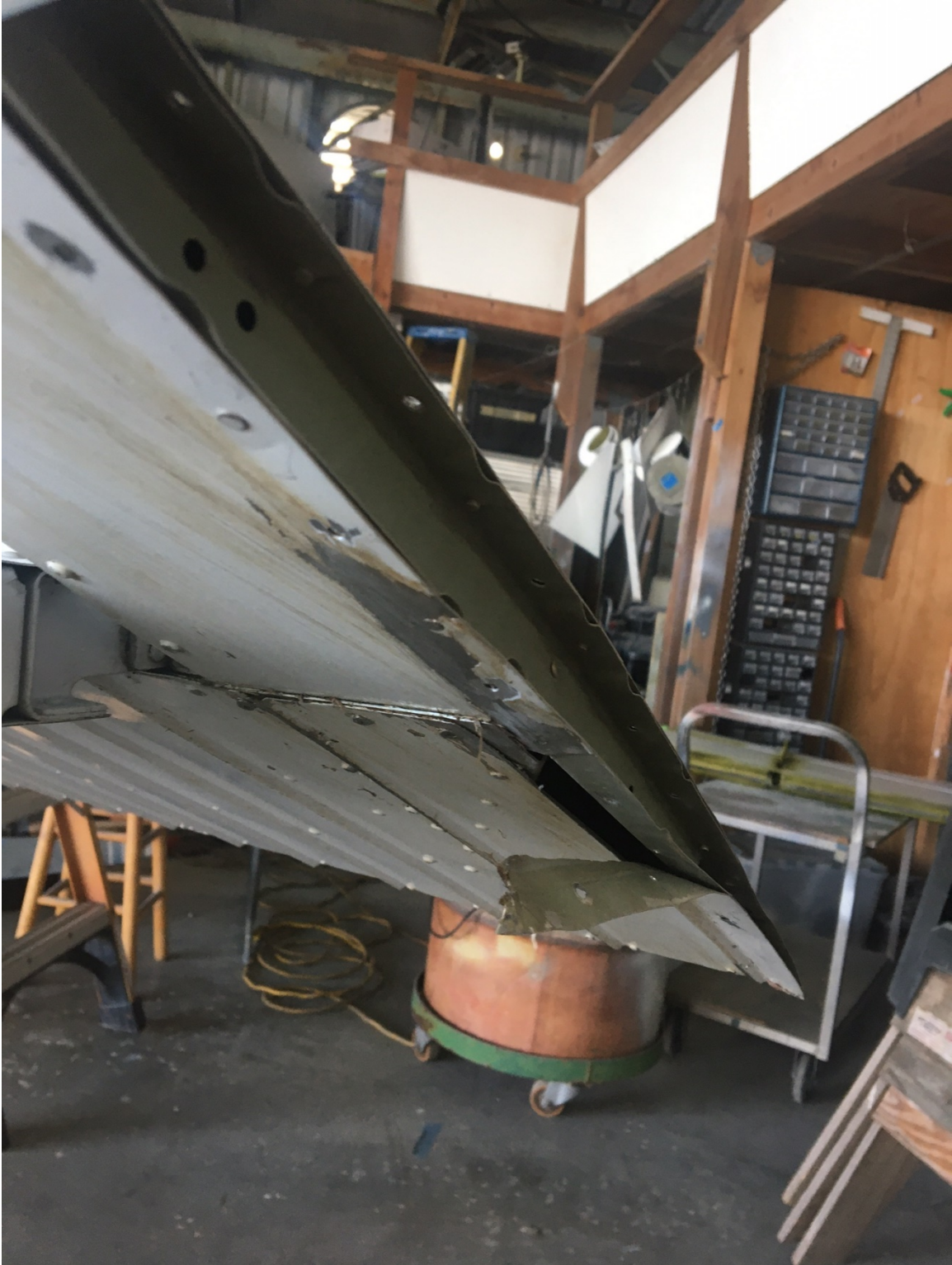
Figure 2 - Damage to Left Side Elevator
