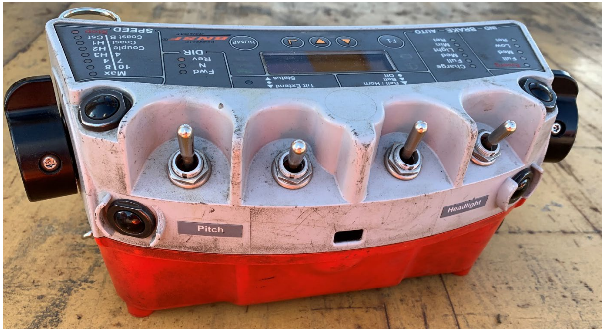
Figure 2. The Switchman Foreman (b) OCU from the accident consist.
