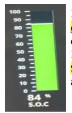
During your pre-trip inspection, make note of your starting <u>State</u> <u>of Charge (S.O.C.)</u> level. This is the current battery-level. Please contact dispatch if it is displaying below <u>50% S.O.C.</u>
