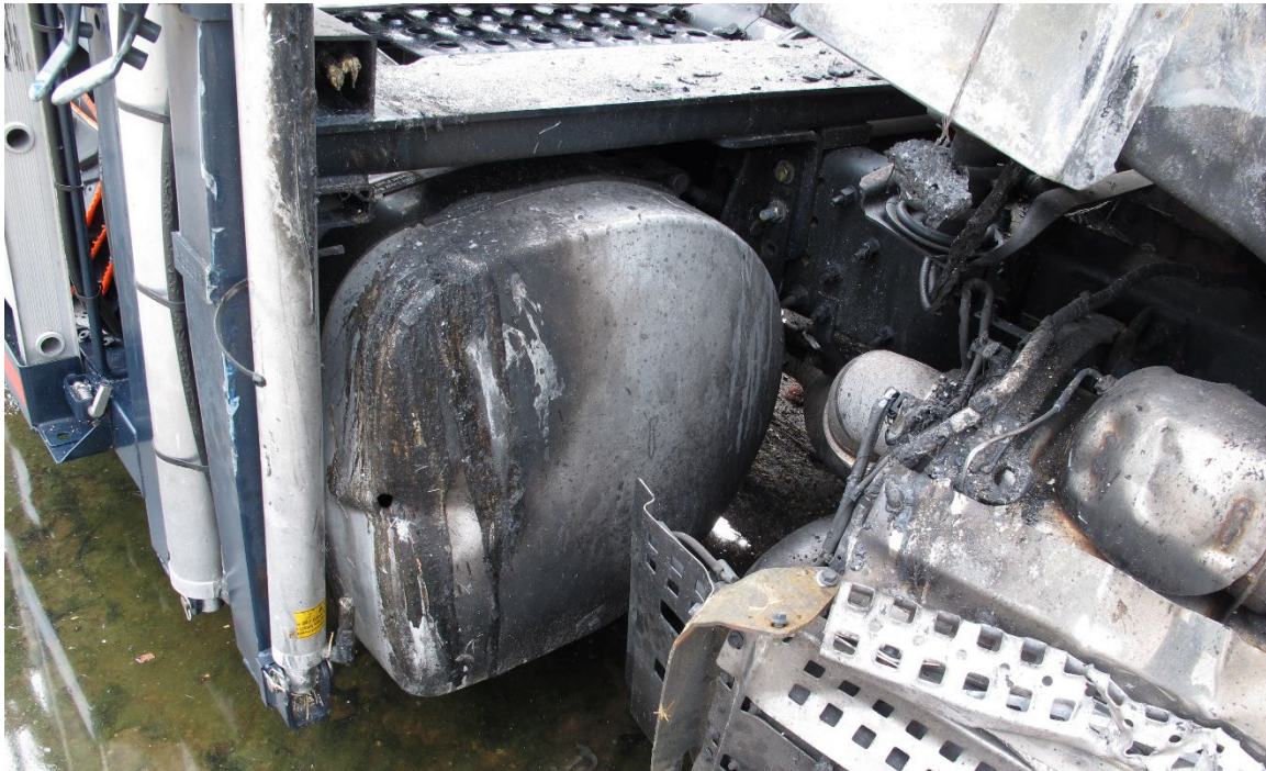
Figure 3. Intact Fuel Tank.
