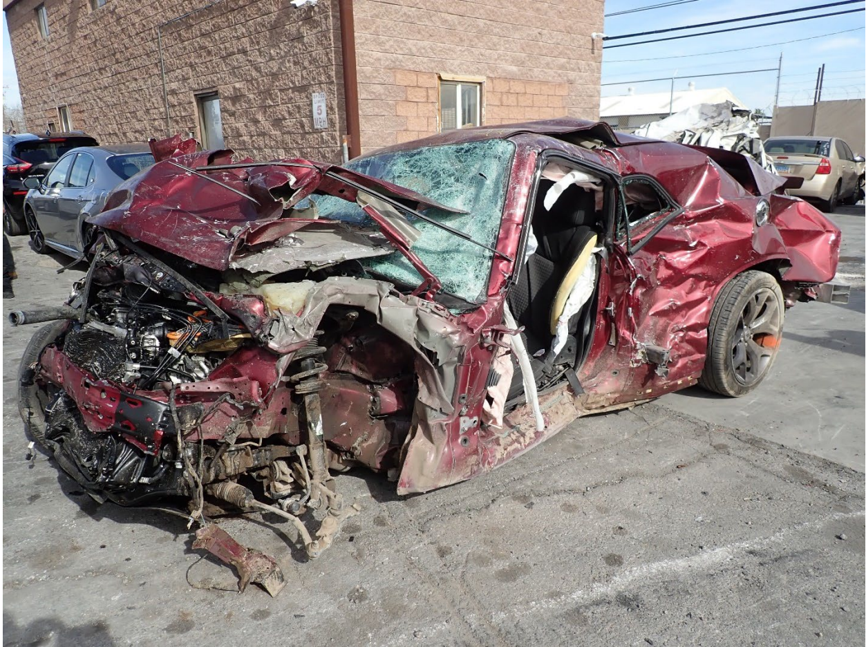
Figure 2. Impact damage to the Dodge Challenger.
