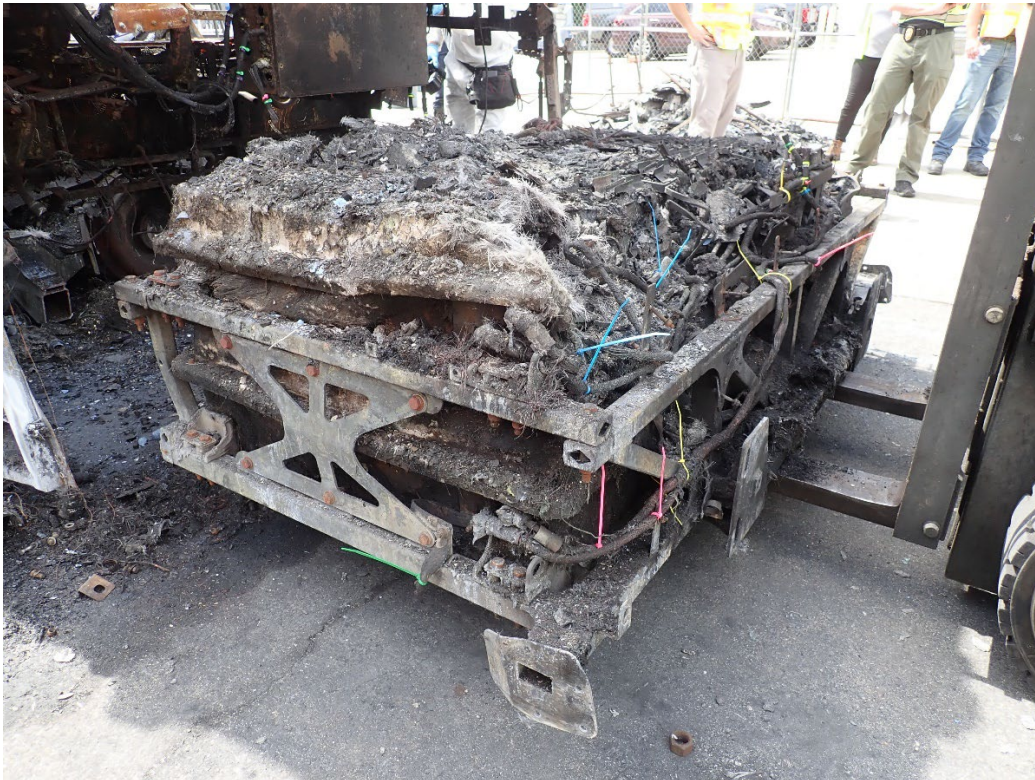
Figure 7: Rear mounted ESS bracket after removal
