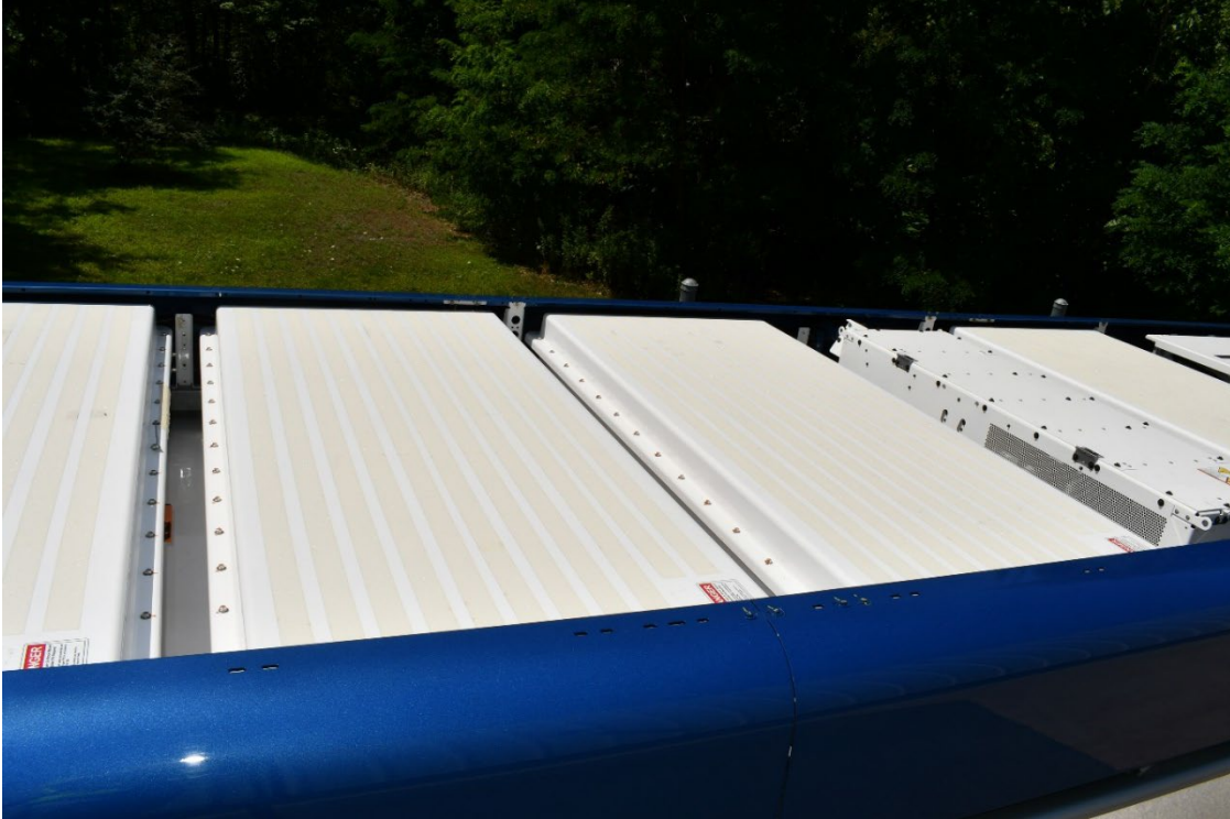
Figure 3: Polyester and fiberglass energy storage enclosures on exemplar bus roof
