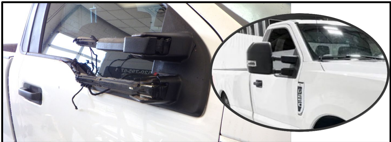
Figure 16: Passenger side mirror damage subject pickup compared to exemplar.
