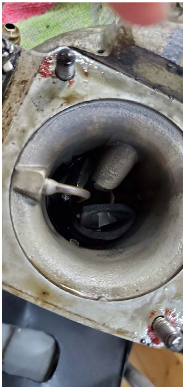
Photo 2 – Carburetor intake. Note the air filter gasket in the throat (Chuck Potts photo)
