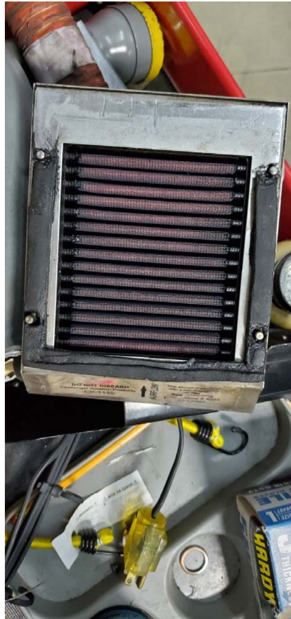
Photo 1 – The condition of the air filter gasket, as found by Chuck Potts, supervising mechanic. Note gasket seal is missing from the top of the air filter (Chuck Potts photo)}
