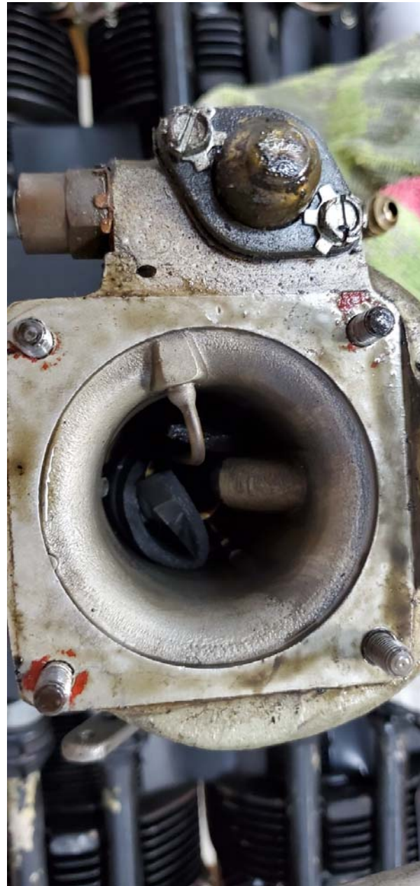
Photo 3 – Another view of the carburetor intake with a piece of the air filter gasket in the throat (Chuck Potts photo)
