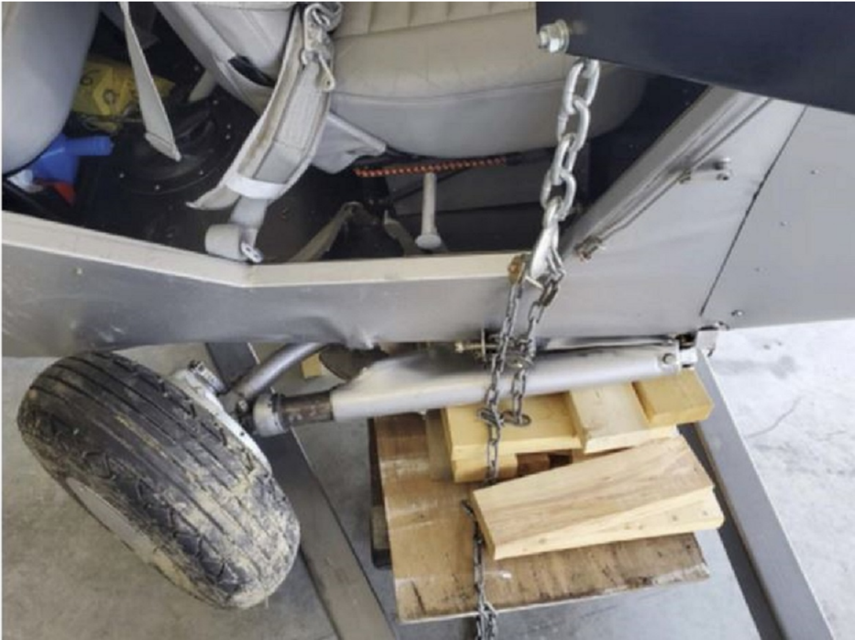
Photo 2 - Buckled right main landing gear (FAA photo)
