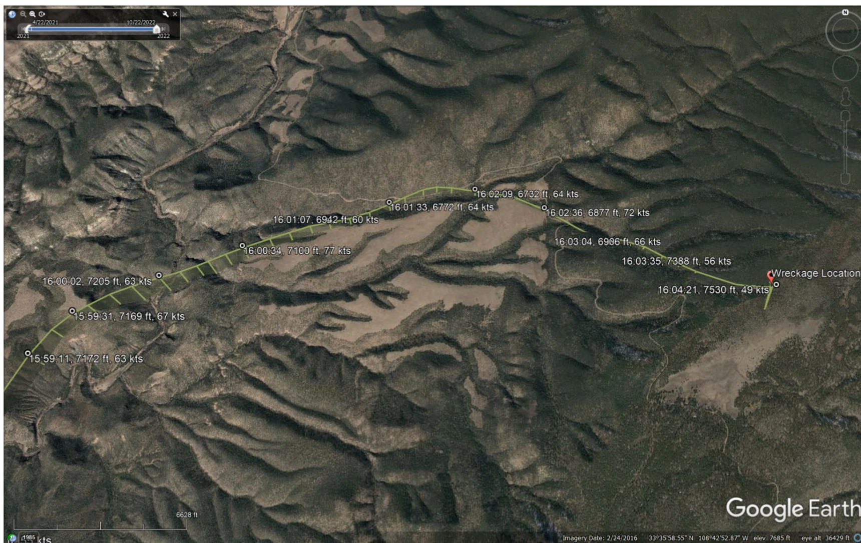
Figure 3. Google Earth overlay showing the final 5 minutes of the accident flight.
