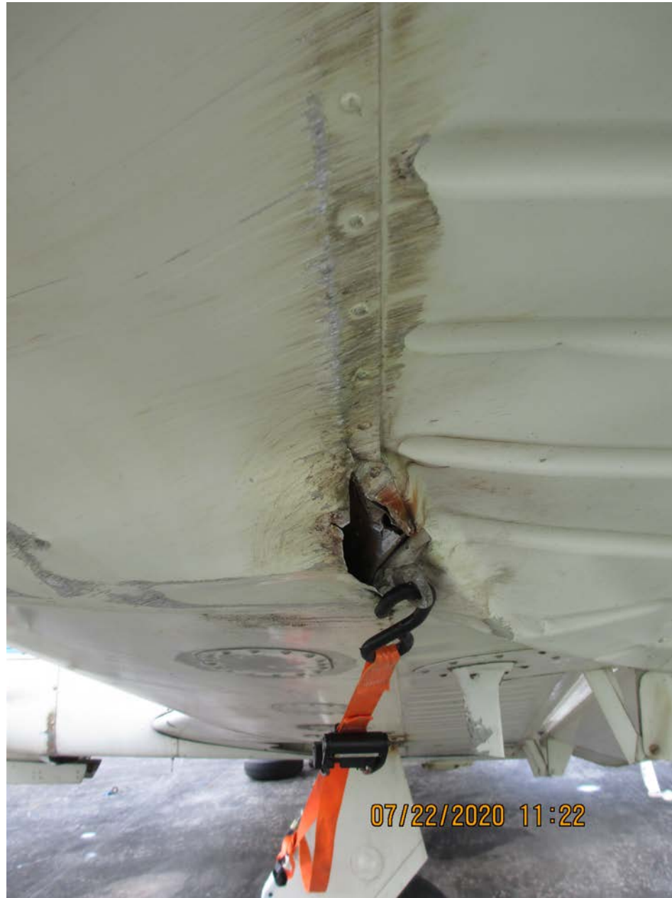
Photo 3 – Right wing and spar damage (FAA photo)
