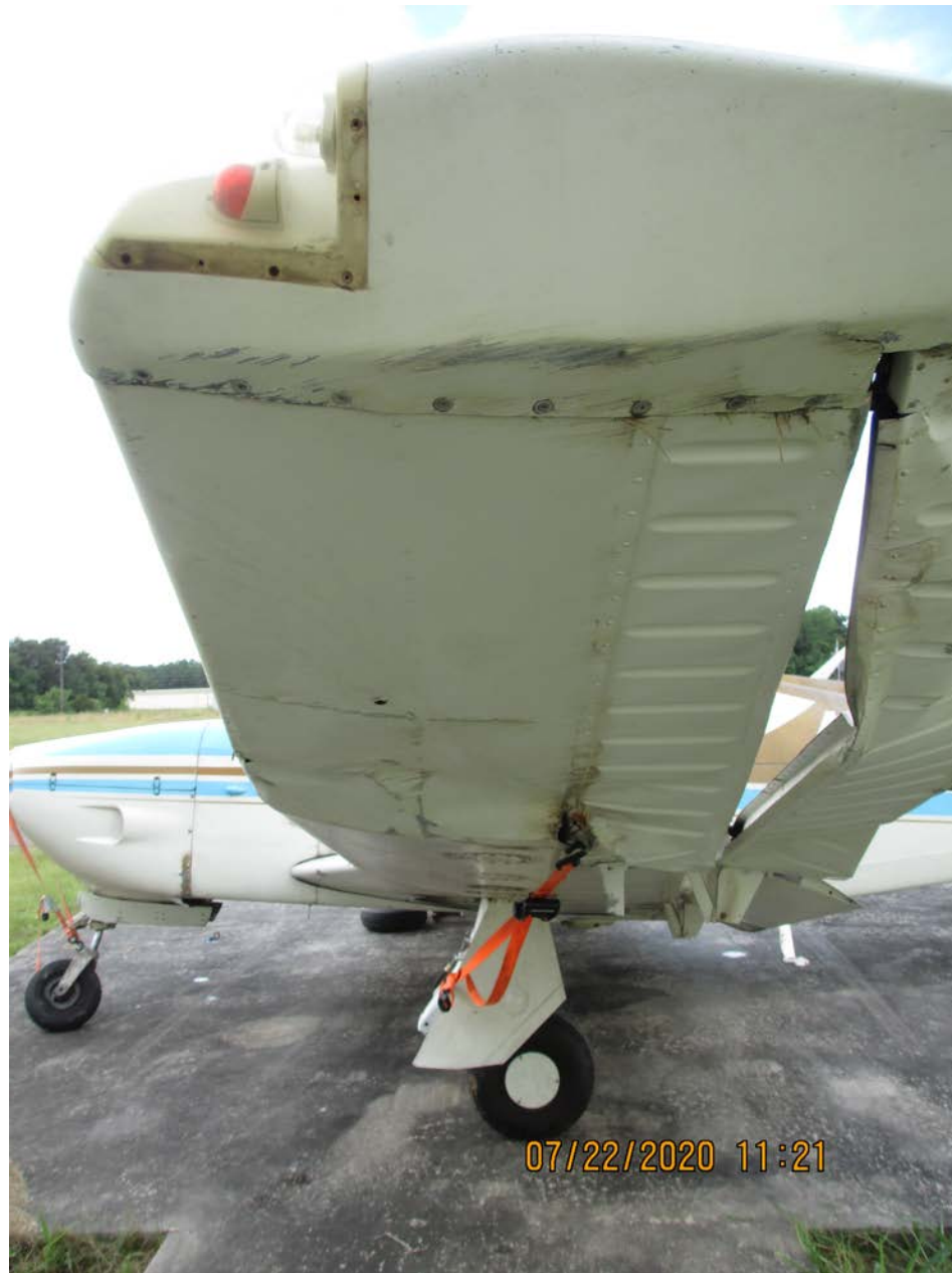
Photo 2 – Left wing and aileron damage (FAA photo)
