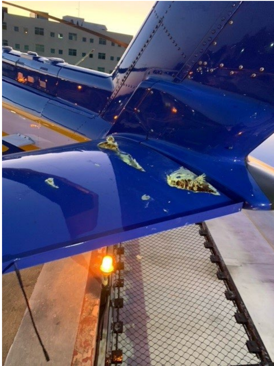
Photo 2 – Fuselage damage - Courtesy of FAA
