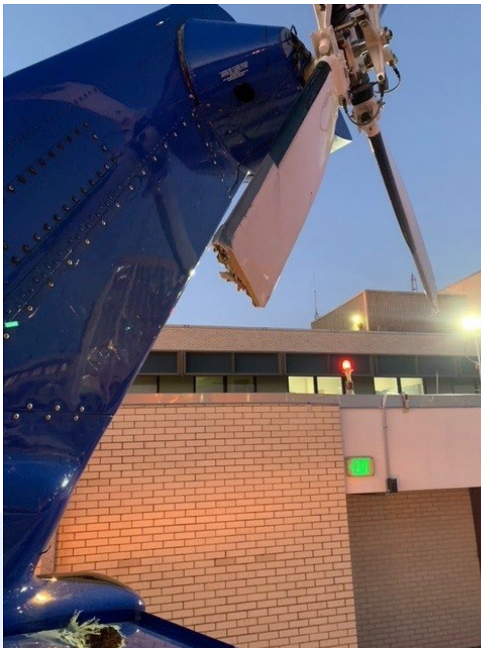
Photo 3 – Tail rotor damage – (Courtesy of FAA)
