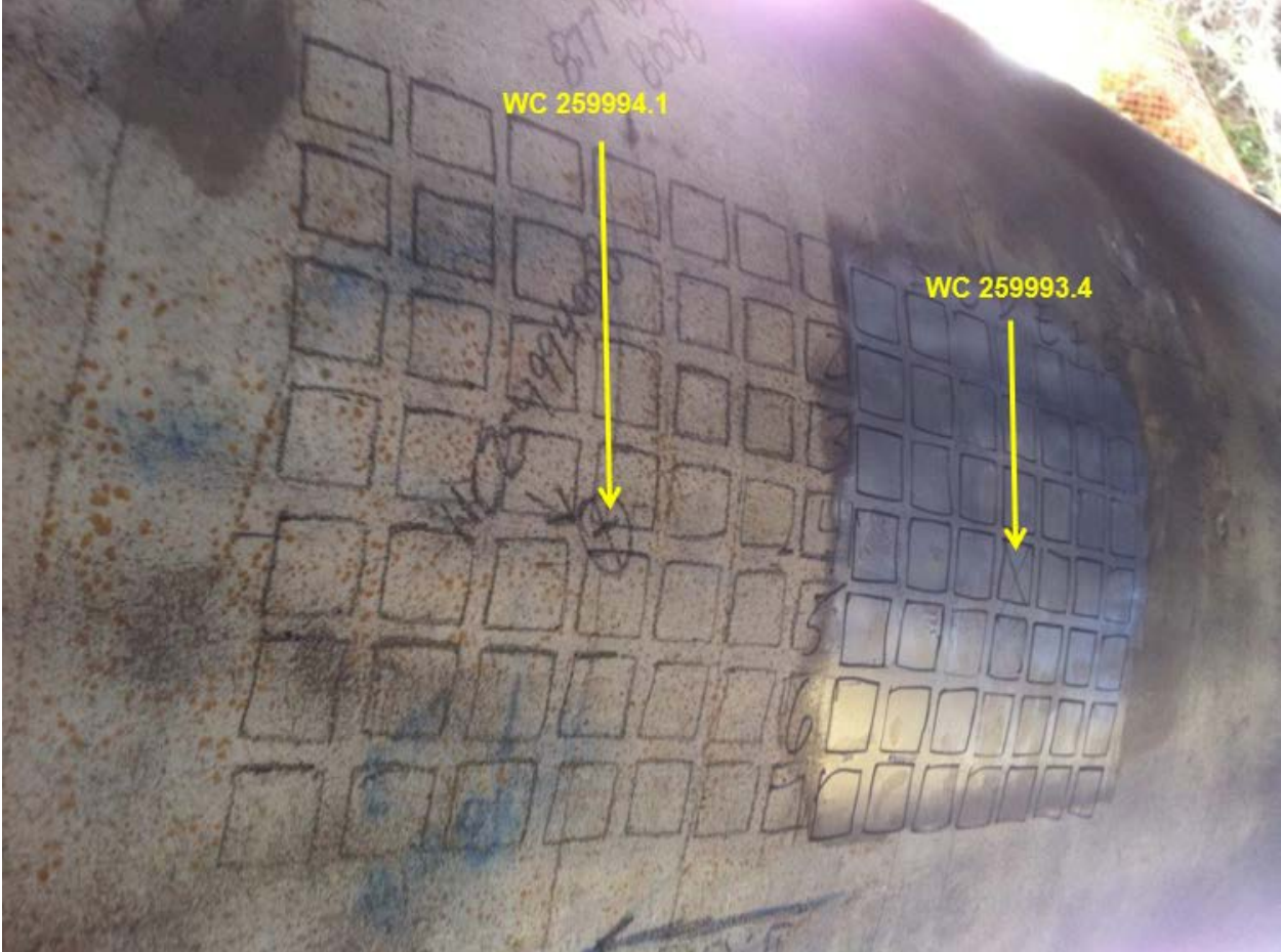
Hard spot test grid for ILI excavation at WC 259994.1 (pre-polish) and WC 259993.4 (post-polish).
