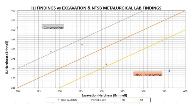
The two non-conservative data points represent the Lincoln County incident origin hard spot. The ILI reported possible hard spot at WC 376895.967 was investigated with polishing and etching at the reported location, however no hard spot was found. It is represented in the table as 0 for metallurgical lab hardness; however the value 0 is not within the scale boundaries of the unity plot.
