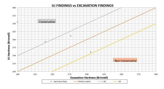
Note: The ILI reported hardness for WC 244877.9 was 355 HB, and the excavation maximum hardness was 160 HB. For Unity plot purposes an excavation hardness of 200 HB was used due to graphing issues.
