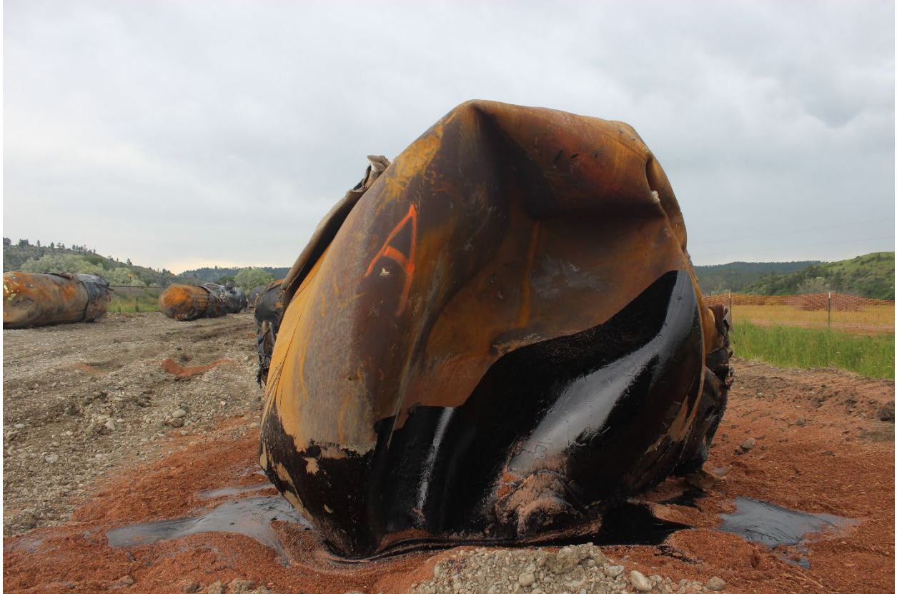
UTLX 644827 B end. The spray-painted A identifies asphalt cars to recovery workers.
