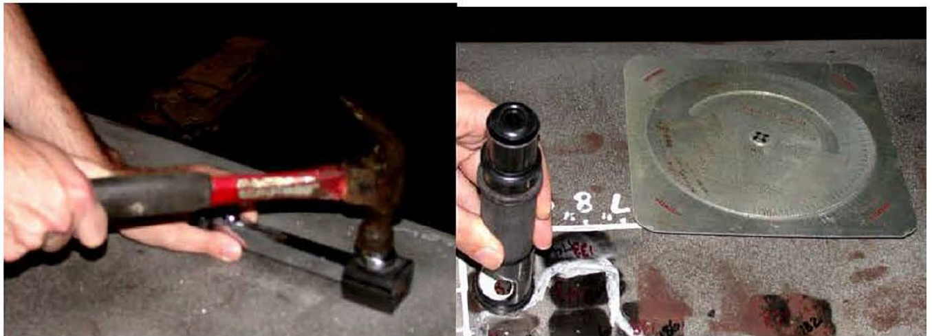
Figure 4. A view of the Telebrineller hardness test equipment. The image on the left shows the bar holder which contains the steel bar of known hardness (280 Brinell), and hammer. The bar holder has a hardened steel ball that creates simultaneous impressions in the pipe and steel bar when the holder is struck with the hammer. The image on the right shows the optical viewer that is used to measure the diameter of the impressions in the bar and in the pipe surface. The calculator is also shown in this image.
