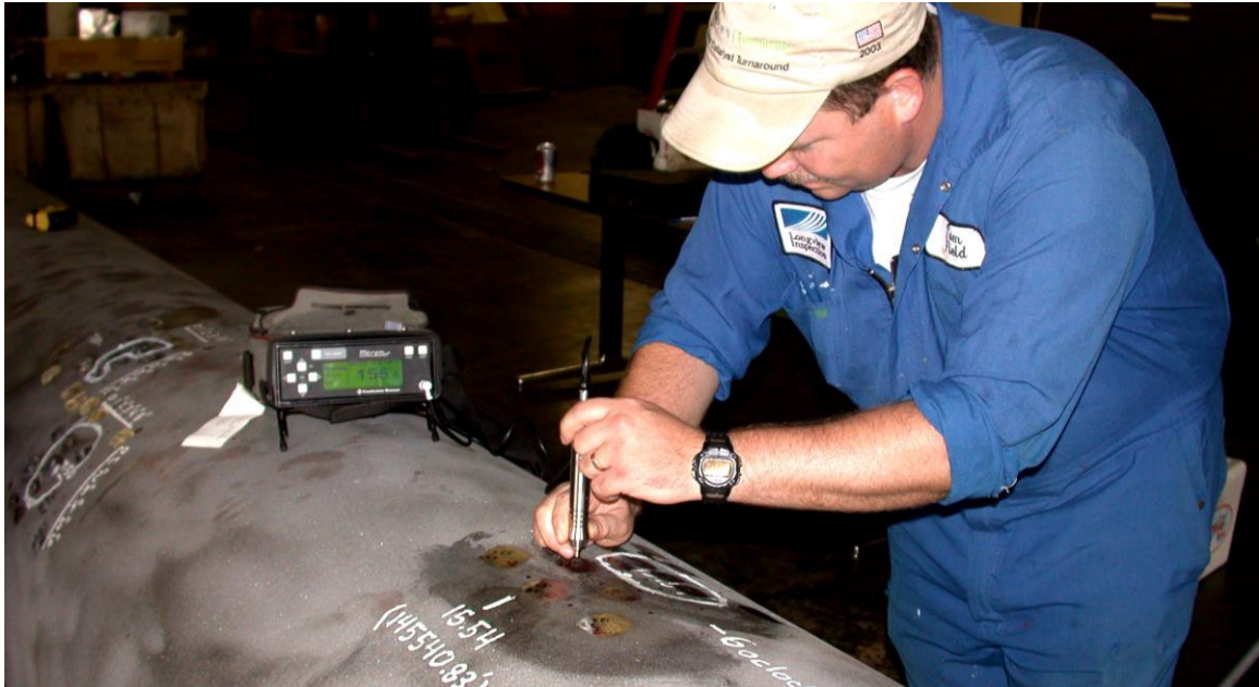
Figure 5. Microdur hardness testing. This method involves ultrasonic contact impedance principles that related the shift in longitudinal oscillation frequency to a Vickers hardness which was converted to Brinell hardness.
