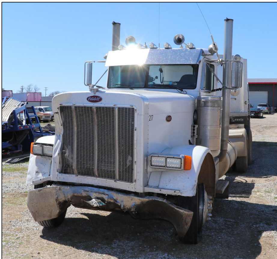
Figure 5: Post-collision photograph depicting damage exhibited by the Peterbilt. Source: NTSB
