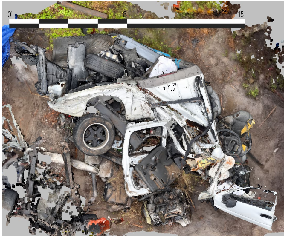
Figure 13. Overhead image of the rendered three-dimensional point cloud depicting the damage to the Chevrolet.
