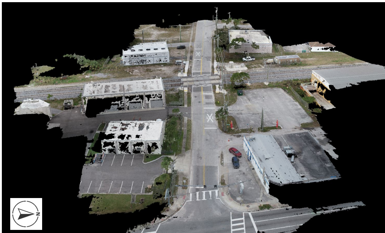
Figure 7. Image of the generated point cloud depicting WH Jackson Street and the highway-rail grade crossing.
