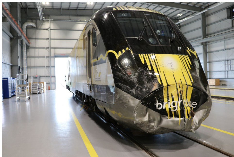
Figure 12. Photograph depicting the damage to the front of locomotive 102.
