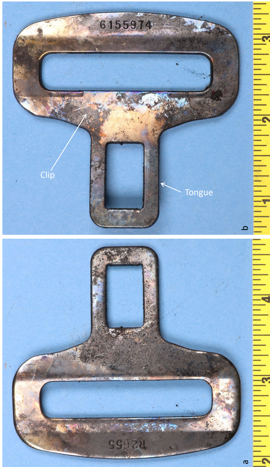
Figure 2 Views of the top and bottom of the seat belt clip with the tongue identified.
