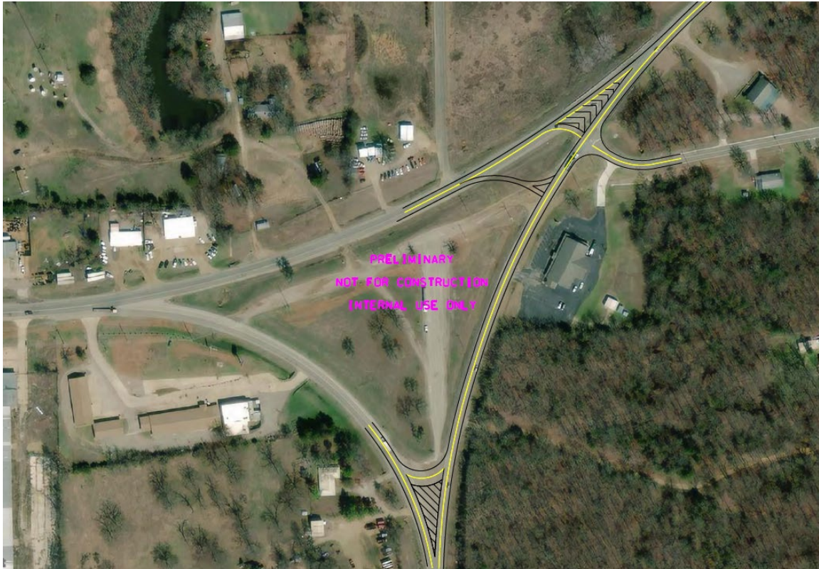
Figure 9. Concept drawing with intersection aligned closer to 90 degrees.
