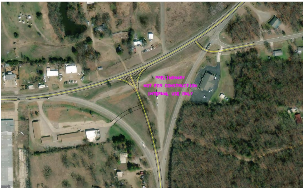
Figure 10. Concept drawing with US 377 routed through the triangle area to intersect SH 22 near 90 degrees.
