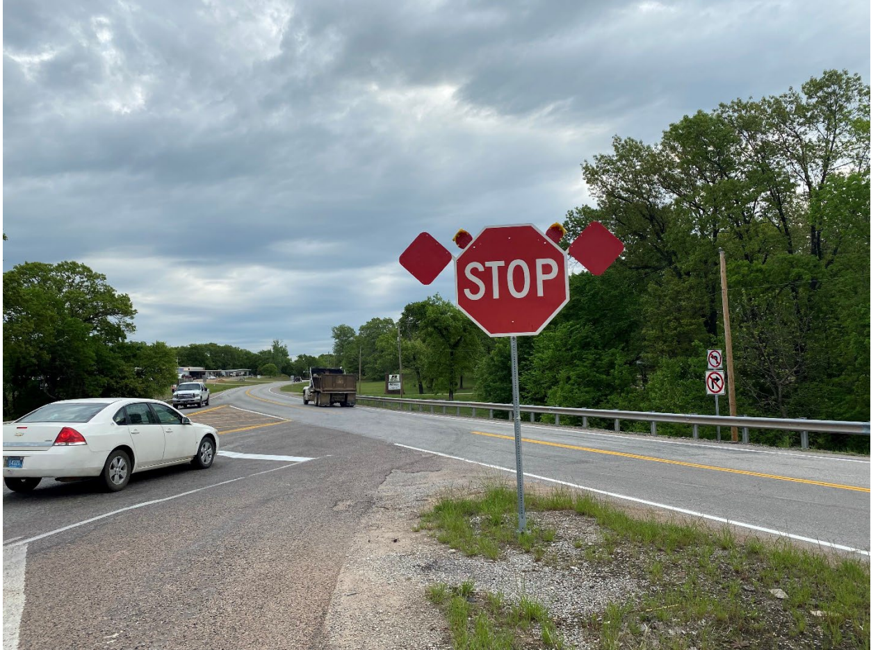
Figure 16. View of STOP sign equipped with flags and flashing beacon at the intersection of SH 22 and US 377. (source: Oklahoma DOT)
