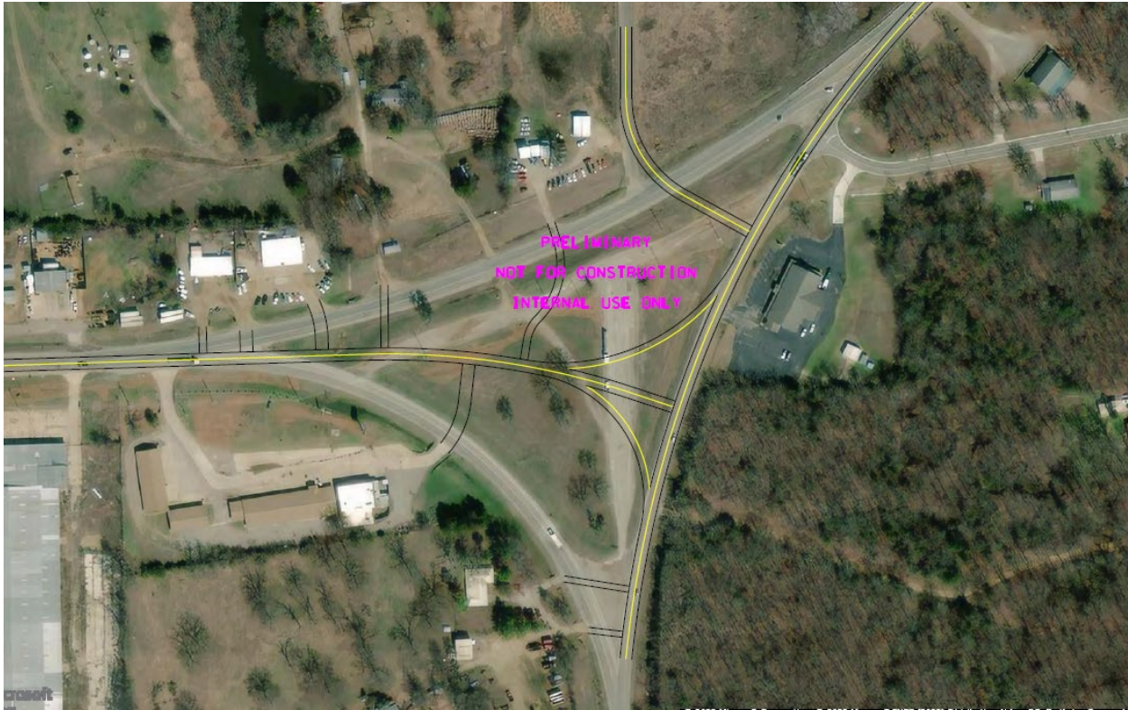
Figure 11. View of concept drawing with eastbound SH 22 re-aligned through the dirt triangle area to intersect US 377 near a 90-degree angle.
