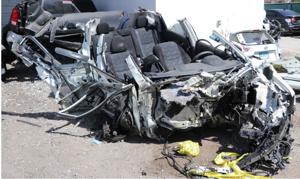
Figure 1. Damage sustained to the right front and side of the SUV.
