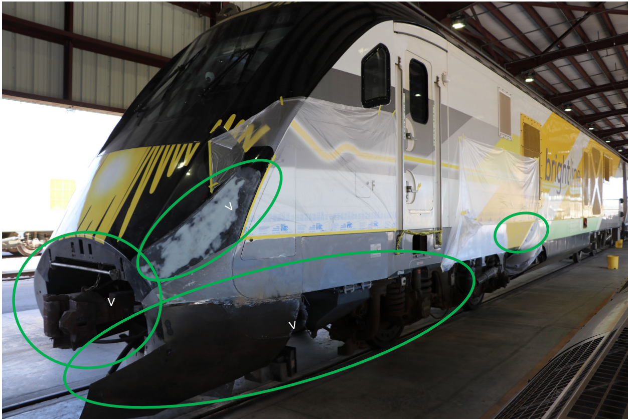
Figure 11. Image showing the left front and left side of crash locomotive. Areas circled in green are areas of repair prior to the inspection.
