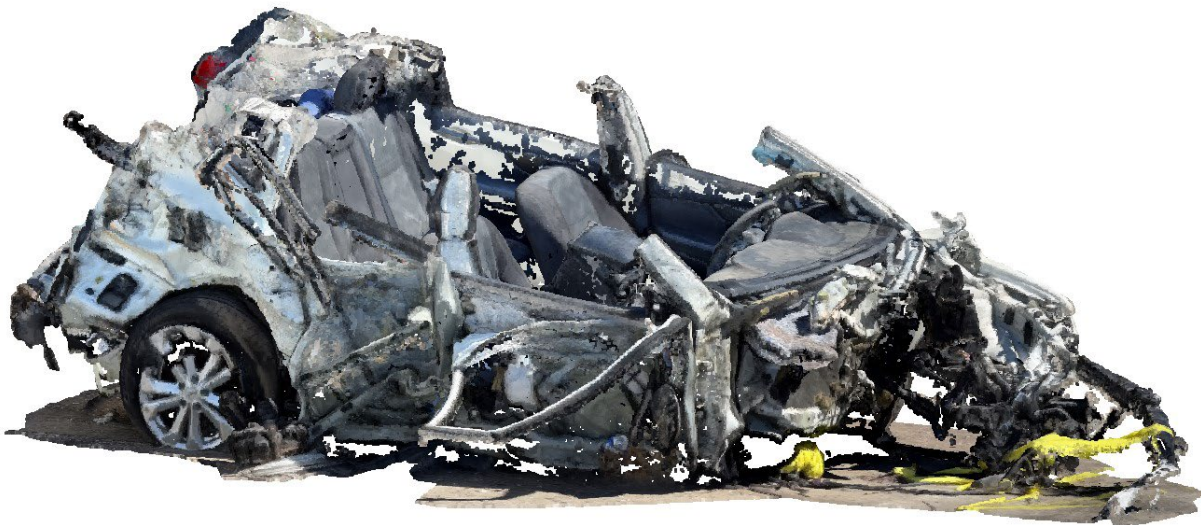
Figure 7. Screen capture image showing 3D point cloud of Nissan as viewed from the right-side of the vehicle. The impact damage to the front is visible.
