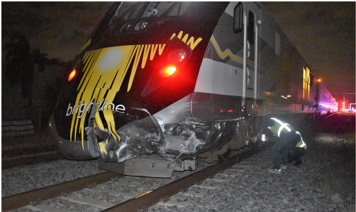
Figure 9. Image depicting damage to the front and left side of the locomotive. View of the photograph is looking northwest. (Source: DBPD revised)
