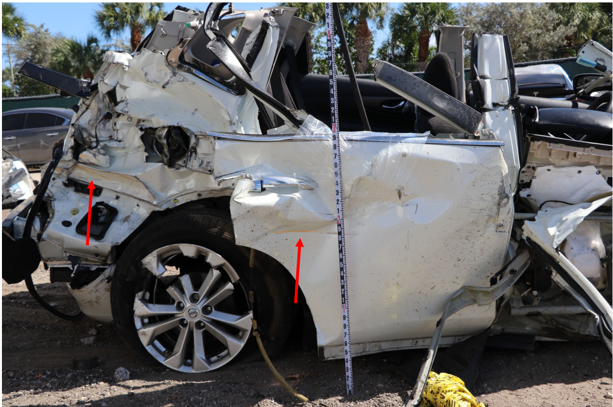
Figure 6. Image of the right side of the Nissan. Red arrows are pointing to the areas of yellow-colored material transfer.
