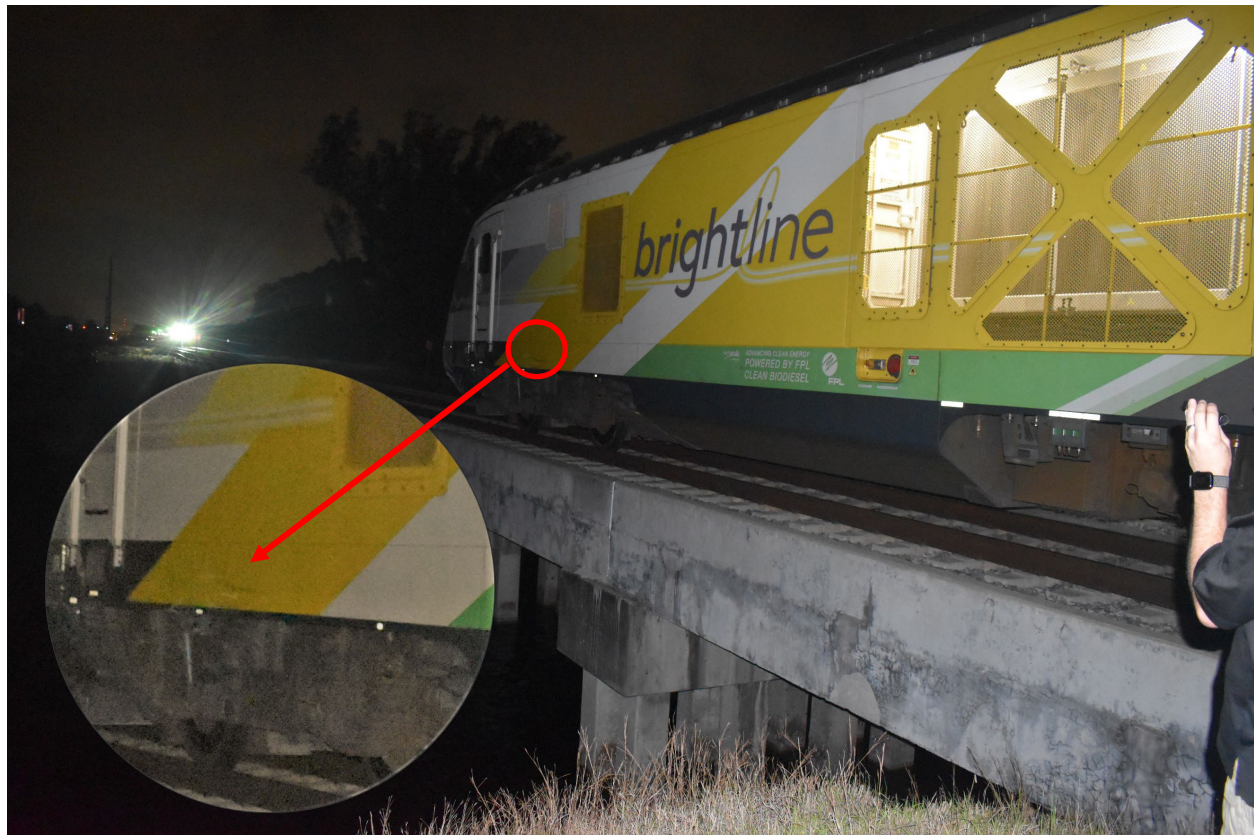
Figure 10. Image of the left side of locomotive looking southwest. Area of second impact circled in red. Inset in lower left corner enlarged image of area circled in red. (Source: DBPD revised)
