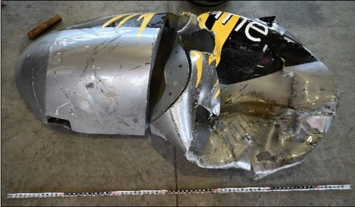
Figure 13: Damaged Nose of the Brightline Train
