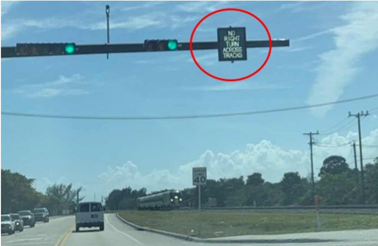
Figure 10 - Hidden Valley Boulevard grade crossing illustrating text only turn prohibition sign indicating "No Right Turn Across Tracks" with the Brightline passenger train shown in the background looking to the south.
