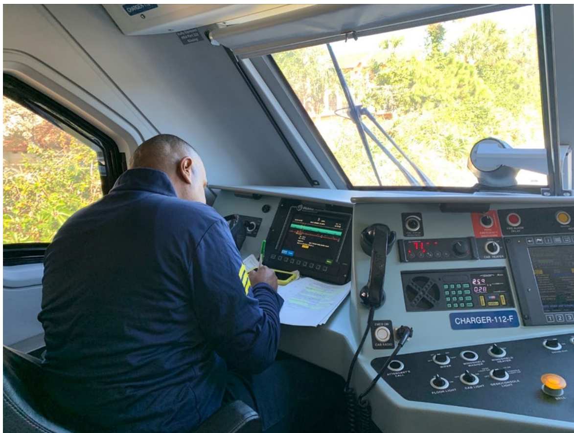
Figure 2. Photograph of an exemplary conductor's station, located on the left side of the locomotive cab, showing a Brightline conductor working.
