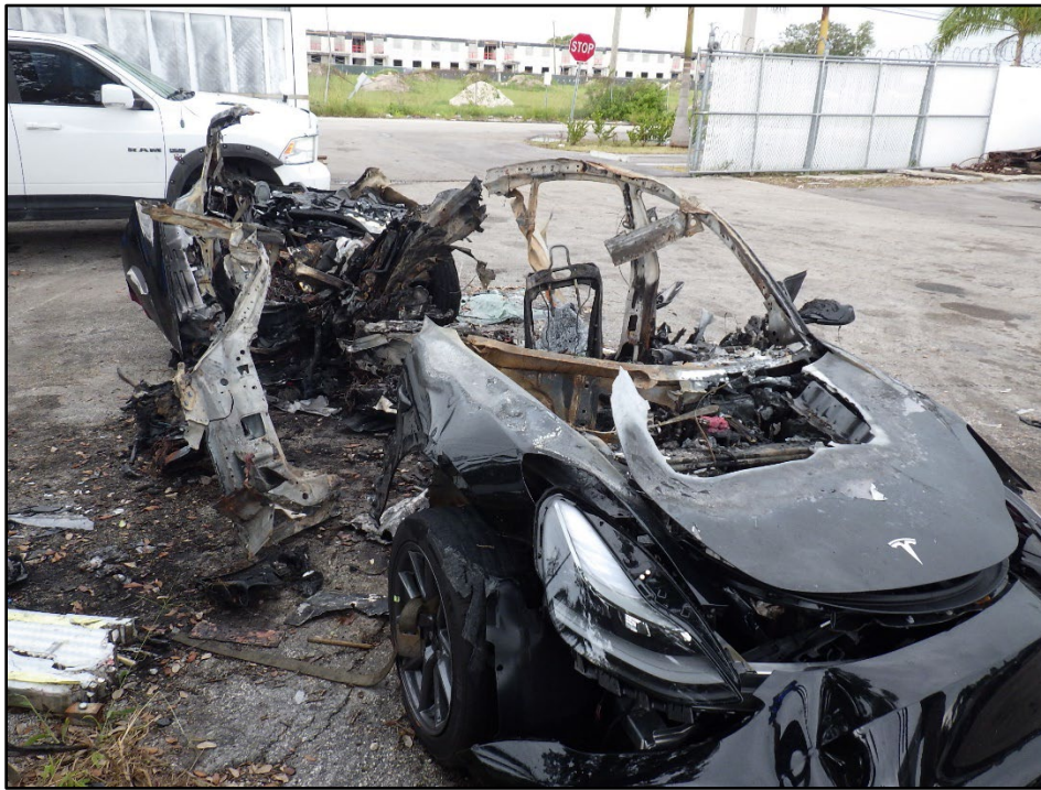
Figure 2. Impact damage to passenger side and fire damage to vehicle interior.
