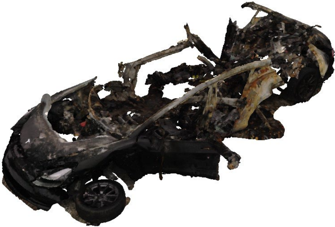
Figure 8: Screen capture depicting the Tesla’s top left side as viewed in the point cloud rendered from the three-dimensional scans through the FARO Scene software.
