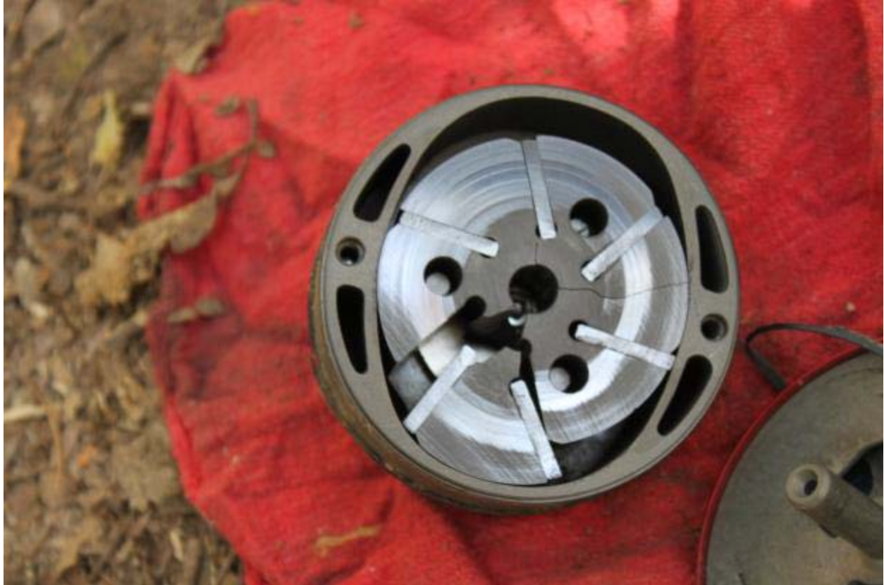
Photo 9: Vacuum Pump After Disassembly
