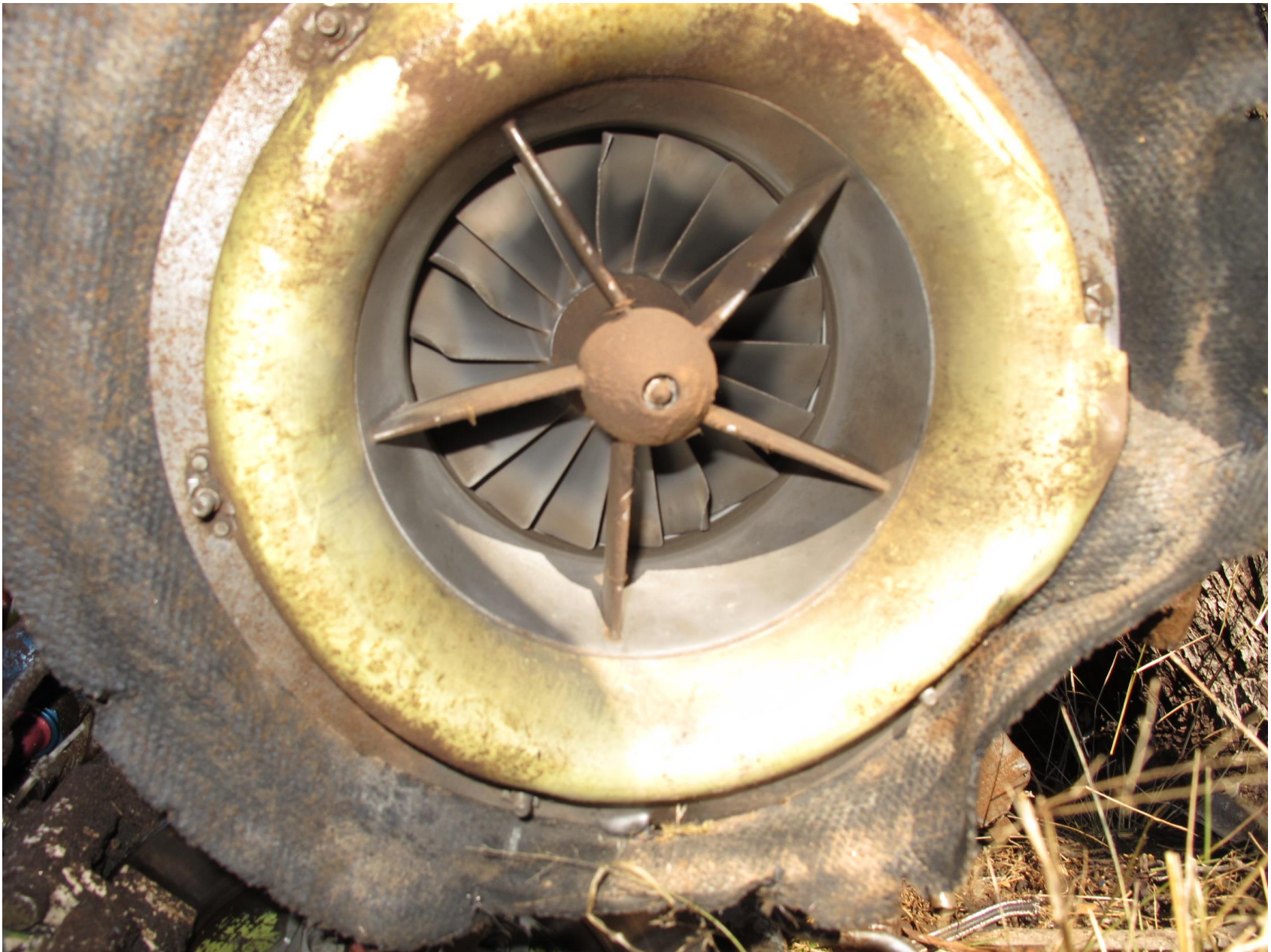
Photo 6 – Engine intake showing compressor blade tips bent opposite to the direction of rotation.
