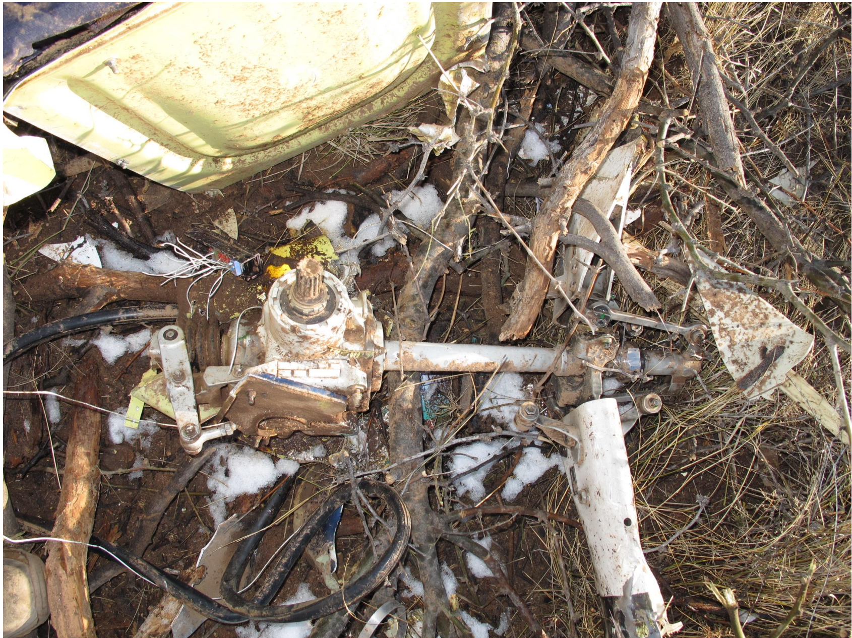
Photo 8 – Tail rotor drive with rotor blades attached to tail rotor hub.
