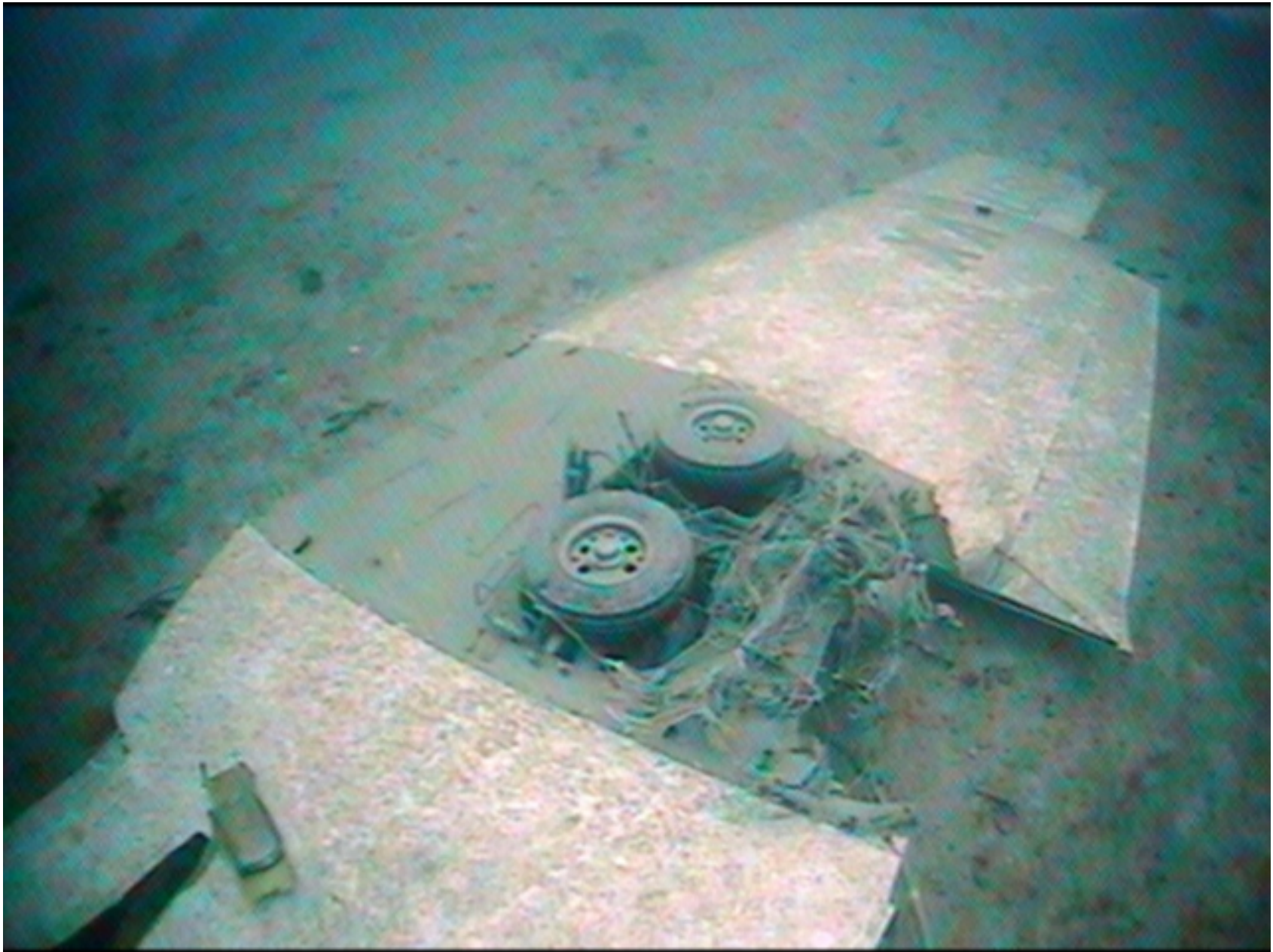
Photo 2 View of Wing, Wing Box Structure, and Main Landing Gear (Salvage Divers)-
