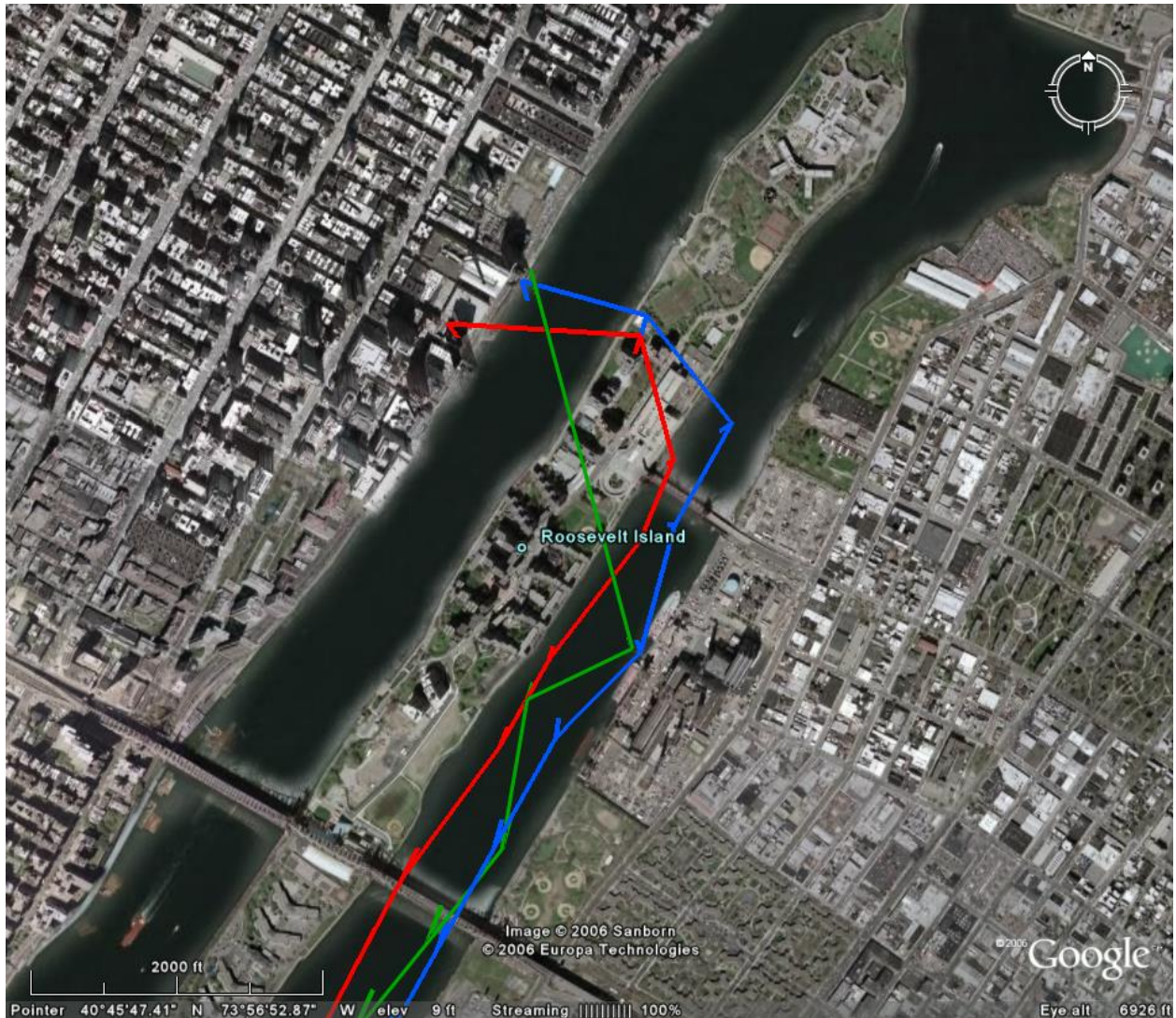
Figure 3: Airplane’s track as viewed by connecting the observed radar targets. Three separate radar sites are plotted. (John F. Kennedy Airport - Red, Newark Liberty Airport – Green, Westchester County Airport - Blue) Please refer to the Aircraft Performance Factual Report contained in the public docket for specific radar and airplane performance information.
