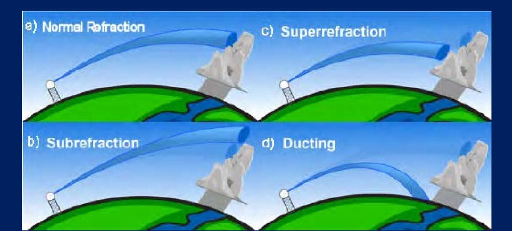
Conversely, sometimes the density of the atmosphere decreases with height at a less than normal rate, or even increases with height. When this occurs, the radar beam will bend more than normal. This phenomenon is called superrefraction
