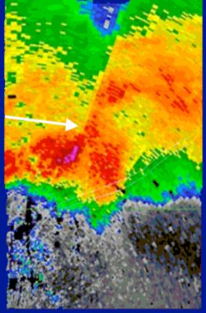
The WSR-88D's 10-centimeter wavelength is not significantly attenuated by precipitation. However, aircraft radars, which typically have 3-centimeter wavelengths, have a significant precipitation attenuation problem. As a result, aircraft weather radar typically only shows the leading edge of extreme intensity echoes.
