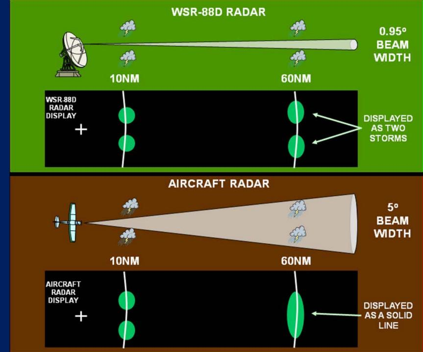
Note that the beam becomes wider at greater distances from the radar. Therefore, the beam resolution decreases with increasing range from the radar. As a result, lines of precipitation may appear to break up as they move closer to the radar. In reality, the breaks in the precipitation were most likely always there
