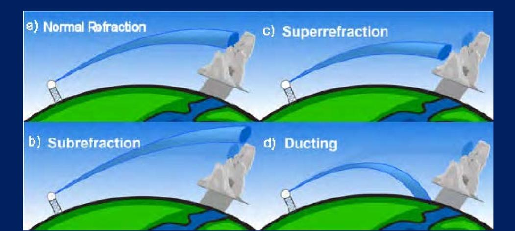
If the atmospheric condition that causes superrefraction bends the beam equal to, or greater than, the Earth's curvature then a condition called ducting, or trapping, occurs
