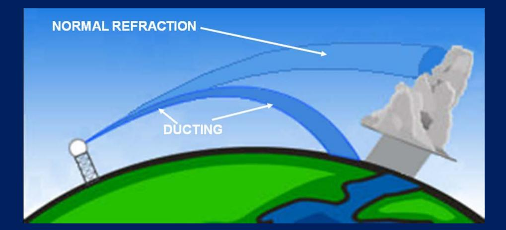
When ducting occurs, the radar beam will hit the surface of the Earth, causing some of the beam's energy to backscatter. This often leads to false echoes, also known as anomalous propagation (AP), to appear in the radar display.
