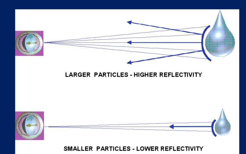
Larger particles have greater reflectivity than smaller particles. For example, a particle with a 1/4-inch diameter backscatters the same amount of energy as 64 particles that each have a 1/8-inch diameter.
