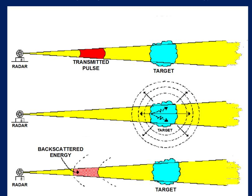
Targets may include precipitation, clouds, dust, birds, insects, buildings, air mass boundaries, terrain features, etc. Reflectivity is a measurement of the amount of backscattered energy. An echo is the appearance, on a radar display, of the backscattered energy
