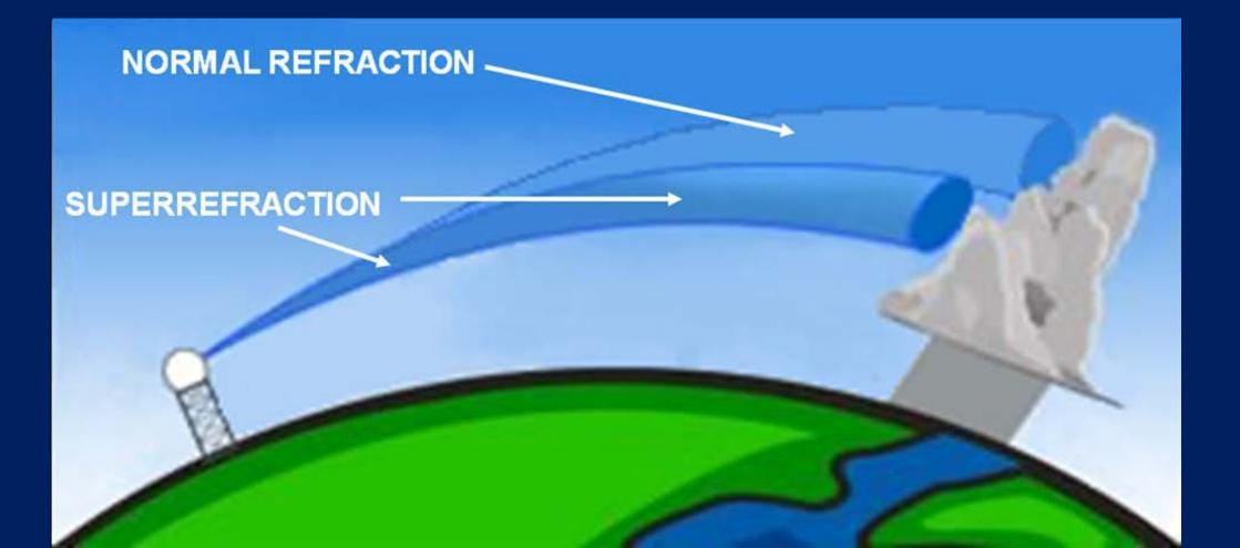
Superrefraction causes the radar beam to travel closer to the Earth's surface than what would occur in a normal atmosphere. This can lead to overestimating the strength of a thunderstorm, as the beam would detect the stronger core of the storm, where precipitation-sized particles are larger.
