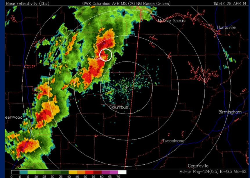
Precipitation attenuation is the decrease of the intensity of energy within the radar beam due to absorption or scattering of the energy from precipitation particles.
