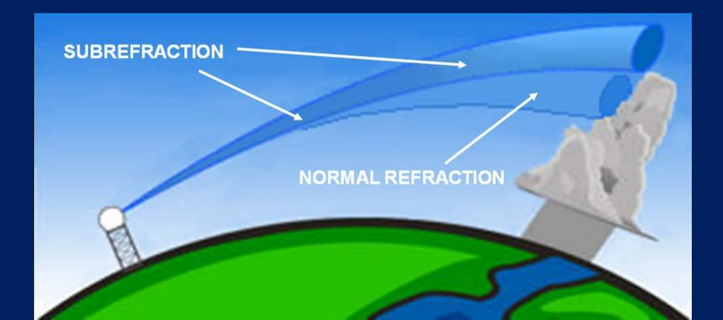
Subrefraction may cause the radar beam to overshoot objects that would normally be detected. For example, distant thunderstorms may not be detected with subrefraction. Subrefraction may also cause radar to underestimate the true strength of a thunderstorm. Thunderstorms may appear weaker on radar because subrefraction causes the radar beam to strike the thunderstorm near the top of the cumulonimbus cloud, where the precipitation particles tend to be smaller
