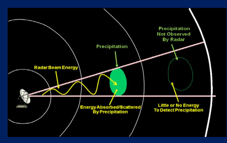
Precipitation close to the radar absorbs and scatters energy within the radar beam. Therefore, very little, if any, energy will reach targets beyond the initial area of precipitation. Because of precipitation attenuation, distant targets (i.e., precipitation) may not be displayed on a radar image.
