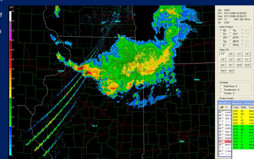
The intensity of precipitation is determined from the amount of energy backscattered by precipitation, also known as reflectivity. Reflectivity is determined by:
