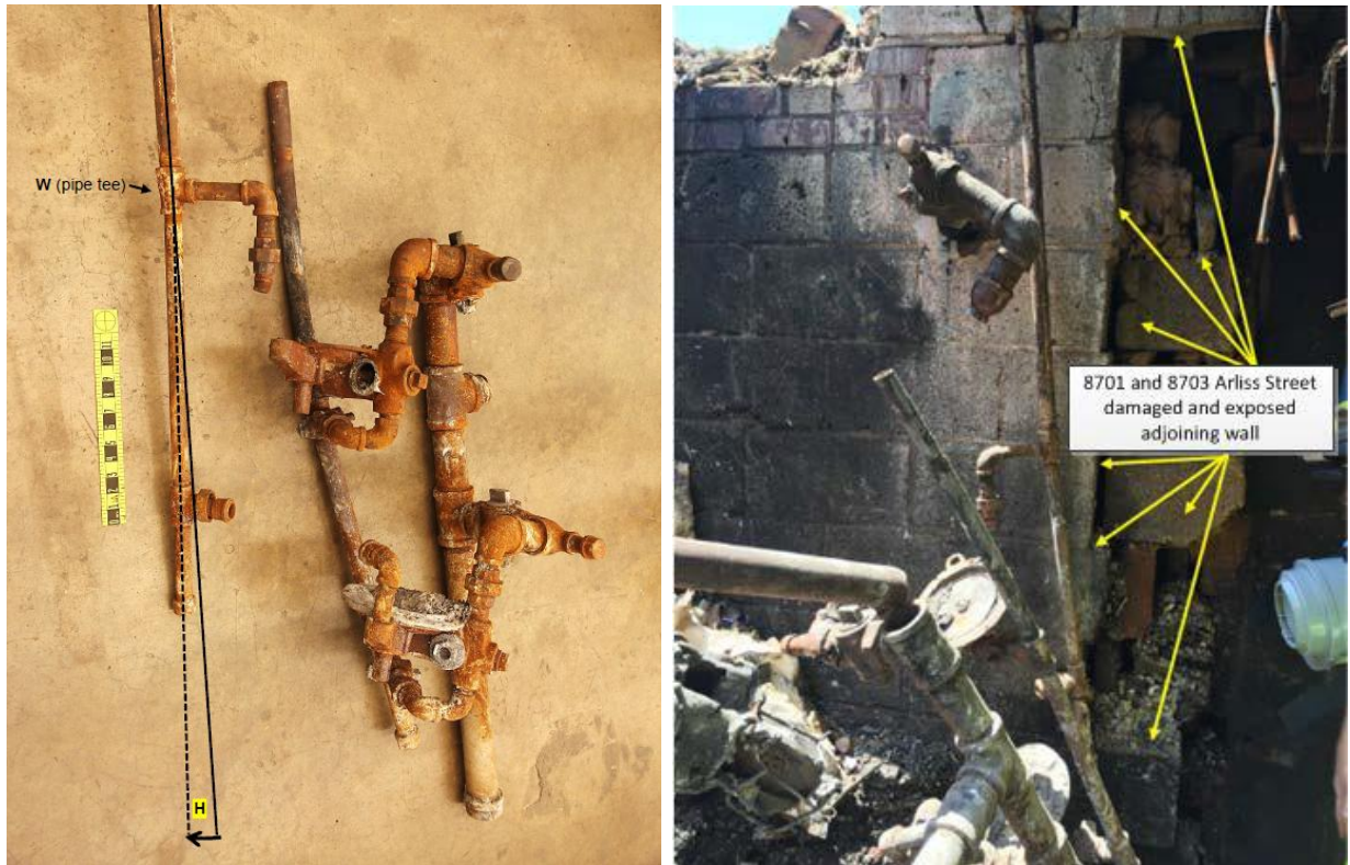
Figure 4A: Bending evident in lower section of vent line
