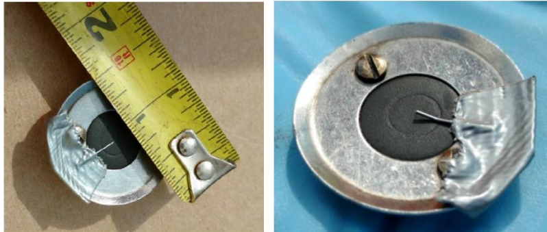
Figure 2. 0.020" Diameter Pin Taped Across Valve Seat (Left). Deformed Pin on Valve Seat, Removed After Regulator Lock-Up (Right).
