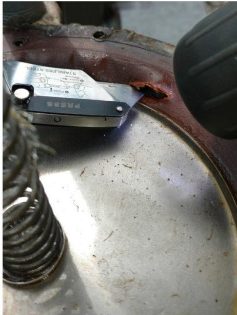
Figure 3. Torn Leather Diaphragm
