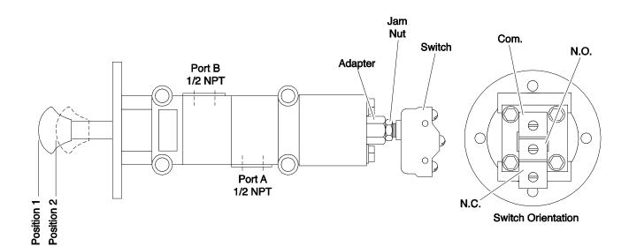
Figure 1 - "D" PILOTAIR Valve Assembly View
