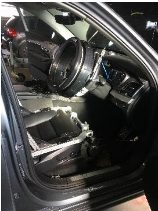
Figure 3: Test vehicle (top), ABD Driving robot install (bottom left), 4a EBT and EPT combination (bottom right)
